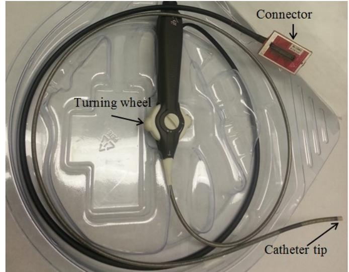
**Figure 6. Completed 64-element Ring array catheter. The shaft handle is shown, on which there is a turning wheel for controlling the pulling wires of the catheter shaft. Also pictured are the custom PCB and connector, used to connect the catheter to the power supplies and imaging system hardware.**
