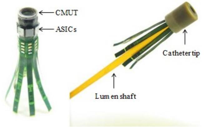
Figure 5. Left: A 64-element Ring array assembly with flex legs folded and adhered with epoxy to the underlying support substrate. Right: Assembly with tip integrated to the flex. The next phase of catheter integration, device encapsulation, has also been completed. Also shown in yellow is the inner lumen shaft.
