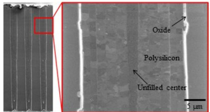
**Figure 2. SEM of the cross-section of a through wafer via.**
