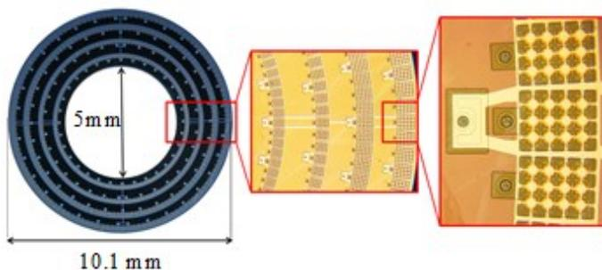
**Figure 1. Optical images of the QuadRing CMUT array. The image on the left shows the entire QuadRing array. The element structure of the four concentric rings and individual elements are shown in the right two images.**
