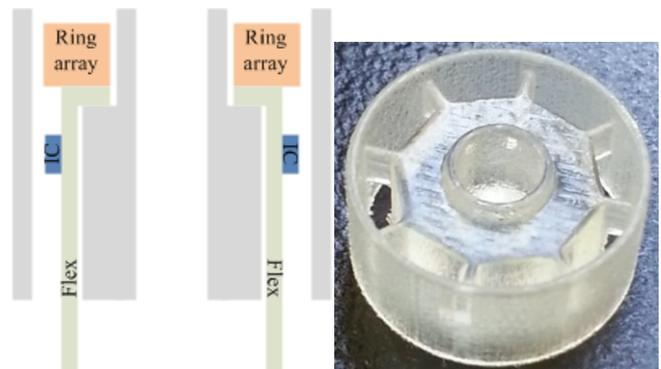
Figure 6. Cross-sectional design (left) and 3D printed tip (right) for the new QuadRing array assemblies. The cross-sectional view shows the flex assembly supported by the inner and outer parts of the structure, as well as the 100 $\mu$ m extension of the structure beyond the CMUT surface. The top-down view shows the octagonal structure of the inner support structure. Each flex leg will be folded through a slit and adhered to one side of the octagon.
