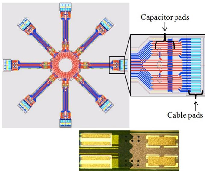
**Figure 3. QuadRing flex design is shown on the top left. The top right image shows the distal end of the flex. The bottom image shows the ridged soldermask edge from a fabricated flex of a previous build.**
