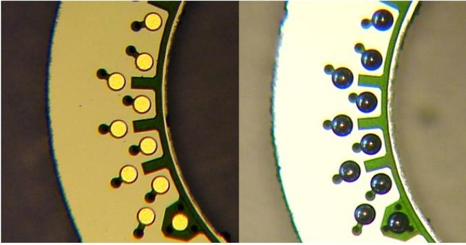
Figure 4. The figure on the left shows the back-side of a 64-element Ring array. The pads and UBM are shown. The figure on the right shows the same type of array, this time with solder bumps on the back-side pads.
