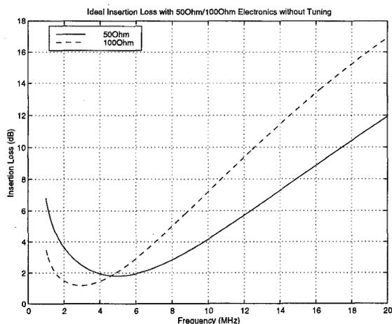
Fig. 9. Ideal immersion cMUT insertion loss.
