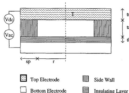
Fig. 1. An immersion cMUT element.
