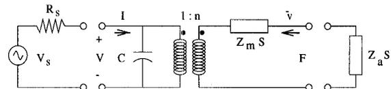
Fig. 4. Electrical equivalent circuit of cMUTs.
