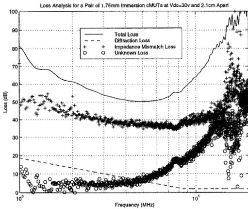
Fig. 5. Total return loss for 1.75mm device.
