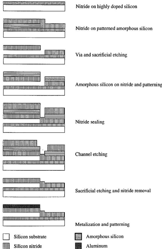
Fig. 2. Fabrication process of cMUTs.
