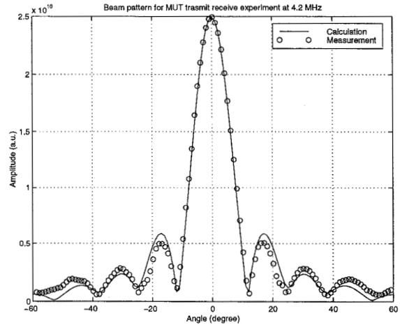
Fig. 7. 1.75mm immersion cMUTs beam pattern at 4.2MHz.
