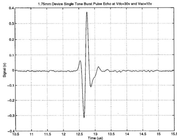
Fig. 6. Pulse echo response for 1.75mm device.
