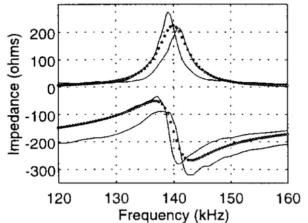
Figure 5: Measured, full lines, and calculated, o o, impedances of test device
