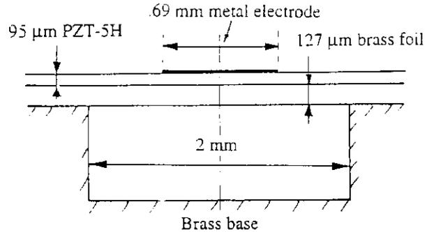
Figure 4: Cross section of test structure
