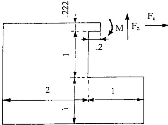
Figure 3. Cross section of support structure for FEM with forces and moment. Dimensions in mm.
