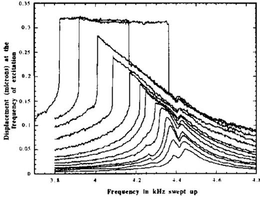
*fig.#5 : Saturation, frequency swept up.*
