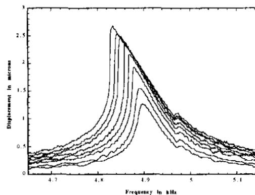
fig.#3 : Resonance frequency drift
