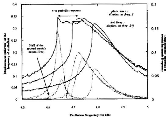
fig.#9 : Non-periodic response due to coupling between the fundamental and the first antisymmetric mode
