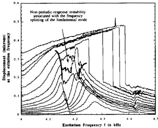
fig.#8 : Non-periodic response due to mode doubling
