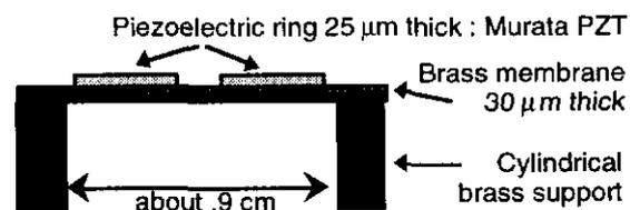
fig.#1 : transducer geometry
