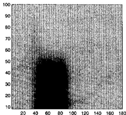
Fig. 8. Image of drilled void in lucite.
