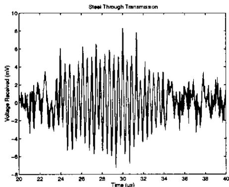
Fig. 6. Air-coupled through transmission of steel.
