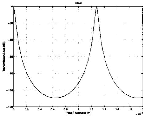
Fig. 5. Loss due to impedance mismatch of steel and air at 2.3 MHz.
