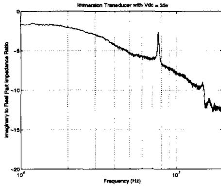
Fig. 9. Impedance ratio of an immersion MUT.
