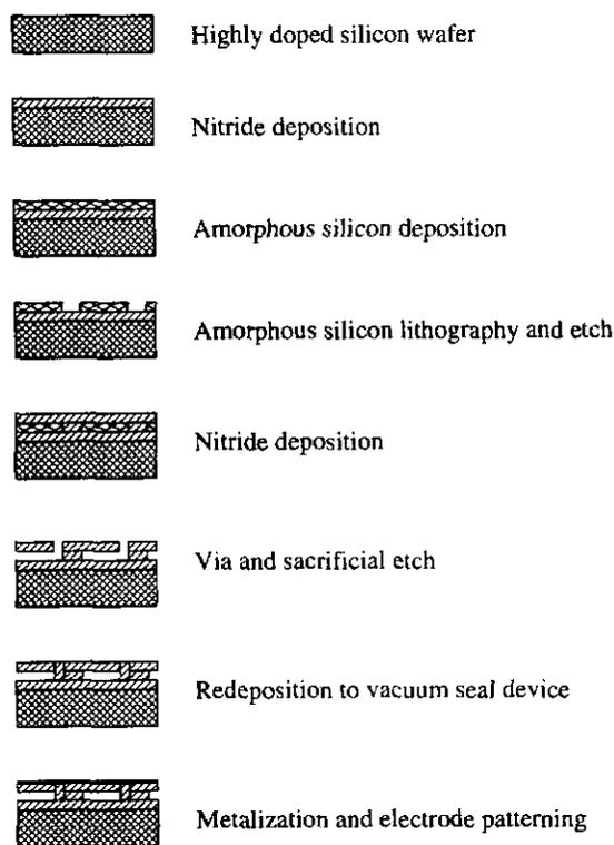
Fig. 2. MUT fabrication process.
