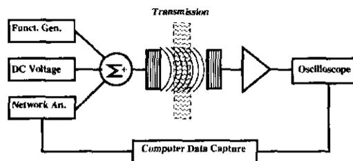
Fig. 3. Schematic of transmission experiment setup.
