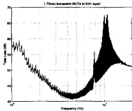
Fig. 10. Two-way insertion loss of untuned MUTs (CW measurement).
