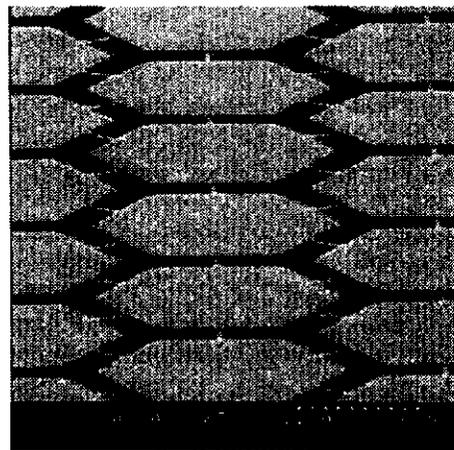
Fig. 1. SEM of a portion of a MUT
