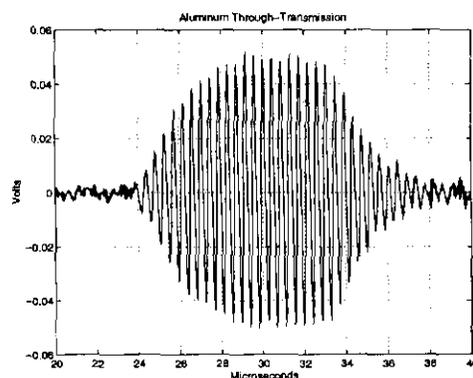
Fig. 4. Air-coupled aluminum through transmission.
