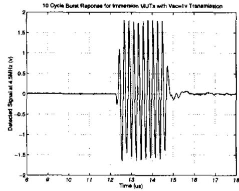
Fig. 11. Transmission of 10 cycle tone burst through oil using MUTs
