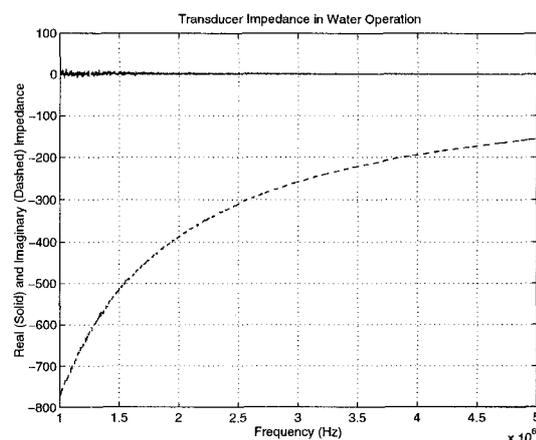
Fig. 9. Transducer impedance with water loading.
