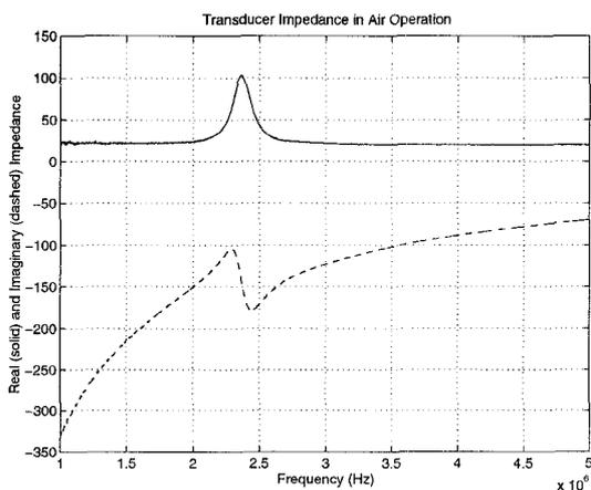
Fig. 7. Transducer impedance with air loading.
