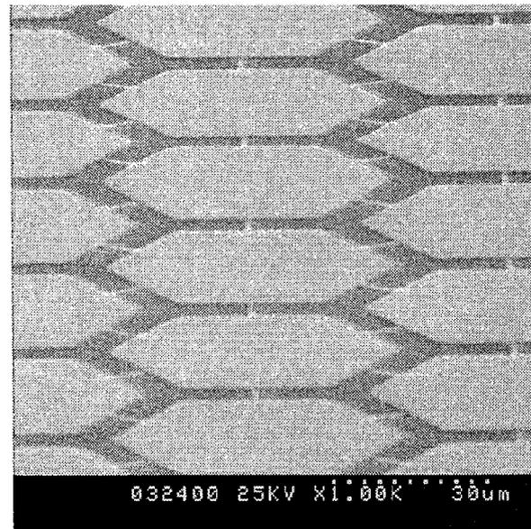
Fig. 6. *SEM top view of the MUT.*
