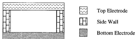
Fig. 1. Schematic of one element of a MUT.
