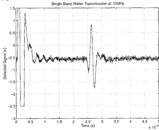
Fig. 11. Single cycle water transmission at 10MHz.
