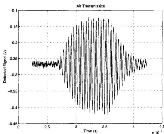
Fig. 8. 20 cycle burst transmission in air at 2.3MHz.
