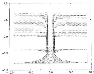
Fig. 4. *SPEEDIE simulation for sealing from bottom.*
