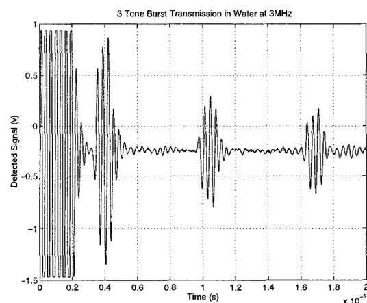
Fig. 10. 3 cycle burst transmission in water at 3MHz.
