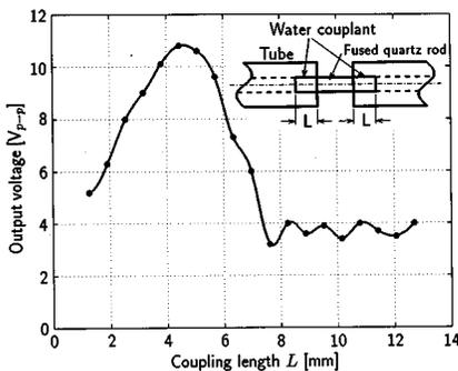
FIG. 5. Variation of transmitted signal intensity for tube-rod-tube configuration.
