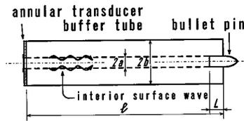
FIG. 2. New configuration of point-contact transducer composed of waveguiding tube and bullet pin.
