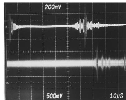
FIG. 7. Signal waveforms obtained for a glass block. Upper trace is at the transmitter and lower one at the receiver.
