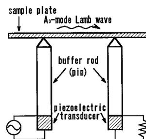
FIG. 1. Time-of-flight measurement system with point-contact transducers.
