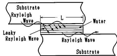
FIG. 4. Mode conversion at two plane boundaries partially filled with water.
