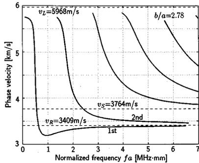
FIG. 3. Phase velocity dispersion curves for symmetric modes in a fused quartz tube for  $b/a=2.78$ .
