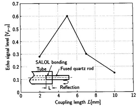
FIG. 6. Variation of the signal intensity reflected back from the rod end. The rod is bonded to the tube with SALOL.
