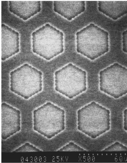
FIG. 2. SEM micrograph of a MUT (top view).
