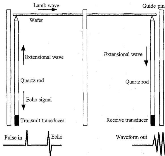
Fig. 4. Set-up for the acoustic temperature sensor (ATS).
