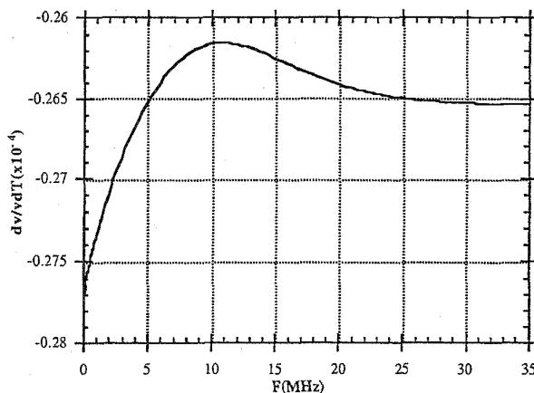
Fig. 3. Relative change in Lamb wave velocity per  $1^\circ\text{C}$  change in wafer temperature.
