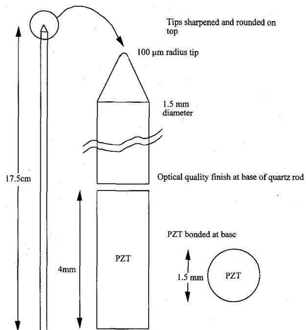
Fig. 7. The transducer pin design for implementation of the ATS.
