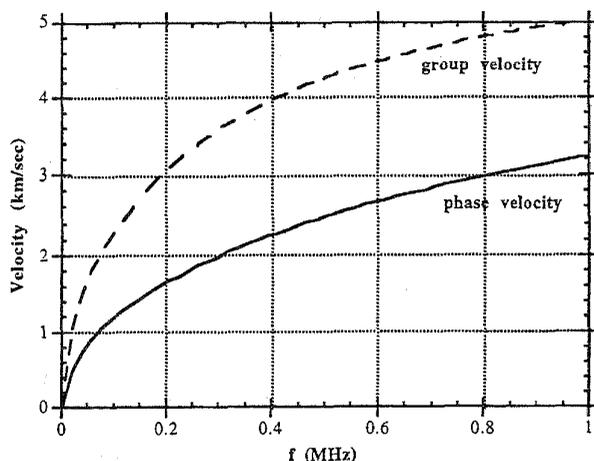
Fig. 2. Zeroth order antisymmetric Lamb wave velocity propagating in a  $500 \mu\text{m}$  (100) intrinsic silicon along the (100) direction.
