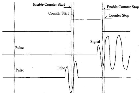
Fig. 5. Timing diagram for deriving time of flight of Lamb wave propagation where the pulse-echo signal is used to start the time interval counter and a specified zero-crossing of the total time of flight signal is used to stop the counter.
