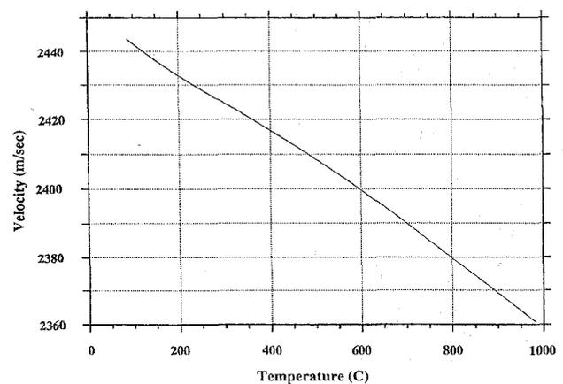
Fig. 10. Regression model of Lamb wave velocity along the (100) direction as a function of temperature.
