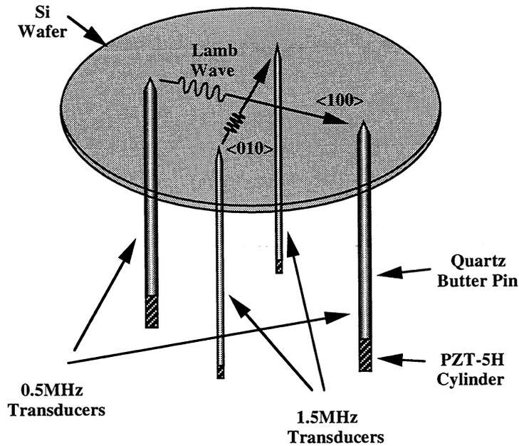
Fig. 3. Experimental setup of the sensor system. Two transmitter/receiver sets are aligned perpendicular to each other along  $\langle 100 \rangle$  and  $\langle 010 \rangle$  direction in order to have the Lamb waves travel effectively on the same crystal axis. The quartz buffer pins are 50mm long with diameters of 3mm for the 0.5MHz transducers and 1mm for the 1.5MHz transducers. The sensors are installed in an IBM aluminum sputtering station in which the experiment is performed.
