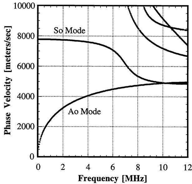
Fig. 1. Phase velocity dispersion relation of a 0.5mm thick silicon wafer along  $\langle 100 \rangle$  direction. We operate at low frequency region where only two modes,  $S_0$  and  $A_0$  mode, can exist.
