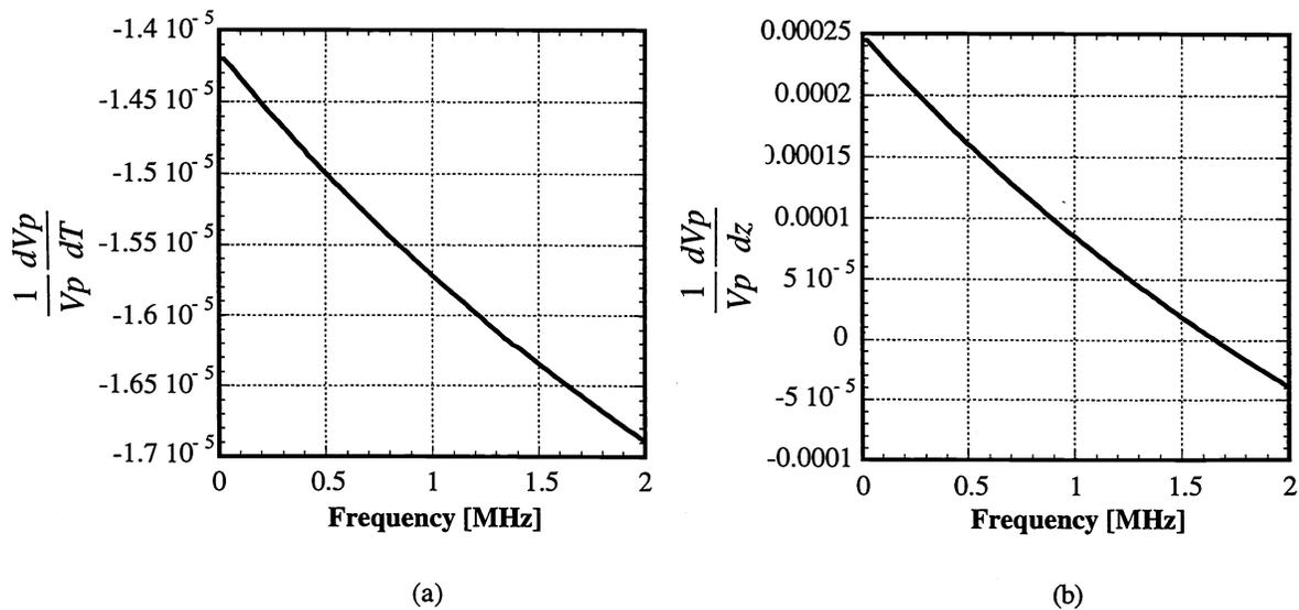
Fig. 2. (a) Theoretical calculation of  $A_0$  mode phase velocity temperature dependency. The fractional change of  $V_p$  due to temperature variation does not change much with frequency. (b) The fractional change of  $A_0$  mode phase velocity as  $1\mu\text{m}$  of aluminum film is deposited on a silicon wafer. The film dependency varies significantly with frequency. The zero crossing at about 1.6MHz implies that the phase velocity does not change as aluminum film is deposited.
