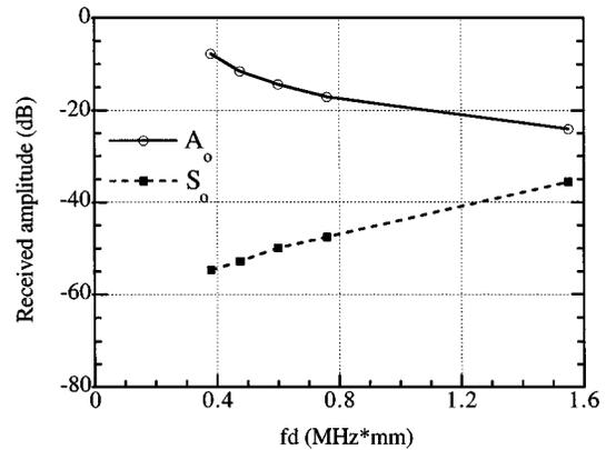
FIG. 3. The measured  $A_o$  and  $S_o$  mode signal amplitudes as a function of  $fd$  for Hertzian contact transducers used in the configuration of Fig. 2(a). The normalization is the same as in Fig. 1.
