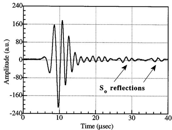
FIG. 5. Digitized output signal when the transmitter and receiver are used in the configuration of Fig. 2(c). The same signals except the  $A_o$  mode signal are observed as in Fig. 4.
