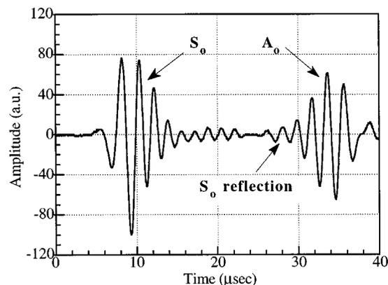
FIG. 4. Digitized output signal when the transmitter and receiver are used in the configuration of Fig. 2(b) and a high voltage spike is applied to the transmitter. The  $S_o$  multiple signal is due to reverberations in the sample.
