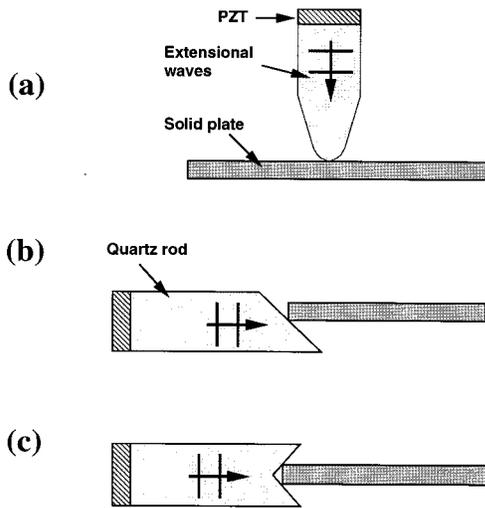
FIG. 2. The Hertzian contact transducer configurations to generate different traction components on the plate surface.
