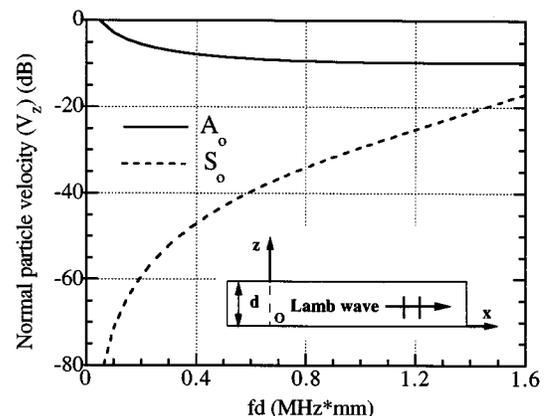
FIG. 1. The normal ( $z$ ) component of particle velocity for the  $A_o$  and  $S_o$  modes excited by a normal traction force on the surface of an aluminum plate as a function of  $fd$ . The inset indicates the coordinate system.
