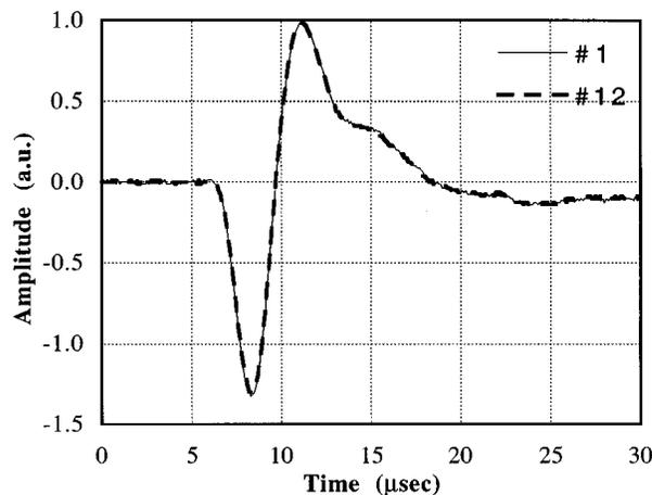
FIG. 7. Probe beam detector output waveforms obtained by the 1st and 12th applications of the Hertzian contact transducer with the probe distance of 2.5 mm.
