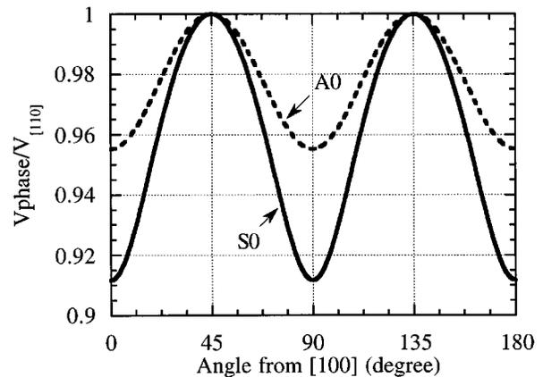
FIG. 4. Variation of normalized phase velocity of lowest order Lamb waves in (001) silicon plate,  $fd=0.056$ .
