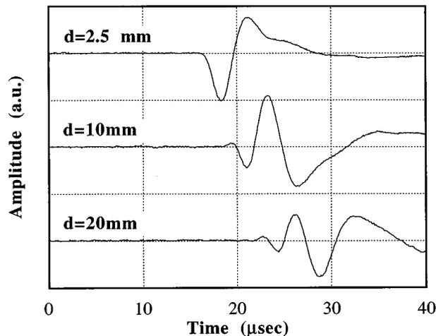
FIG. 6. Optical probe beam detector output for three different spacings between the probe point and the Hertzian contact in  $\langle 110 \rangle$  direction. The sample is a 0.5-mm-thick (001) silicon plate. The signals for  $d=10$  mm and  $d=20$  mm are two times magnified.
