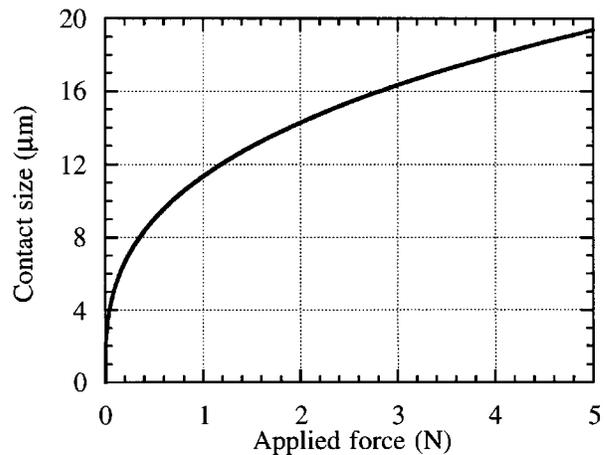
FIG. 2. Radius of Hertzian contact formed between a fused-quartz sphere of radius 100 μm and a planar silicon sample as a function of applied force. Isotropic elastic constants are used for silicon.
