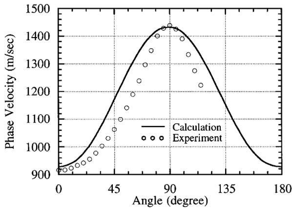
FIG. 11. Phase velocity variation with propagation direction for the A0 mode in the defective region. The angle is measured from the off-fiber axis. The circles represent the measured data and the solid line is the calculated curve.
