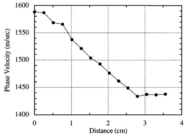
FIG. 12. Measured phase velocity variation data in the fiber direction during the line scan starting in the good region and ending in the delamination region.
