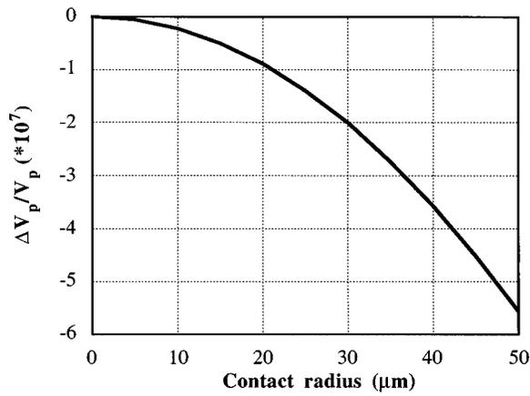
FIG. B1. The normalized phase velocity error due to diffraction as a function of Hertzian contact radius. The error scales with the square of the contact radius.
