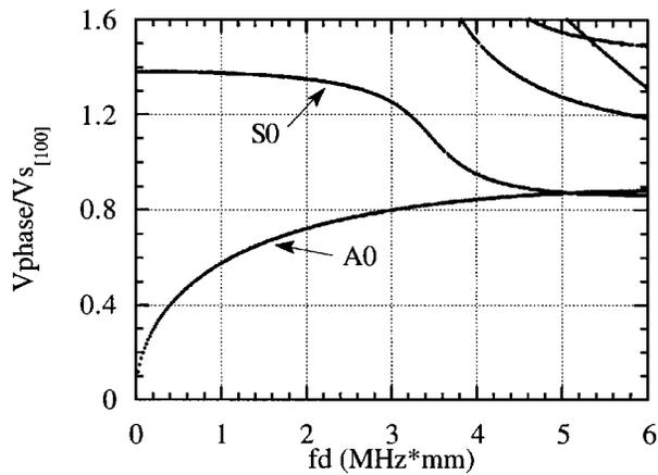
FIG. 3. Dispersion curves for the Lamb wave modes for a (001) silicon plate in the [100] direction. The phase velocity is normalized by the shear wave velocity in [100] direction.
