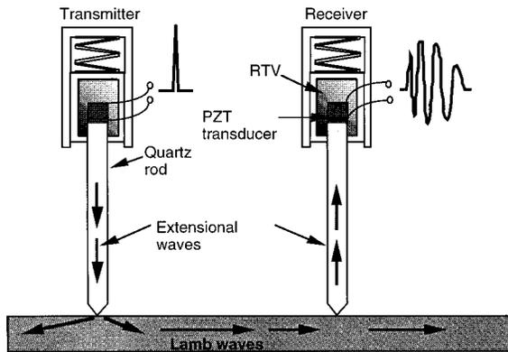
FIG. 1. Schematic of Hertzian contact transducer system with quartz rod and PZT-5H transducer material. The housing is filled with RTV (room-temperature vulcanizing) rubber. The transducers are spring loaded to have repeatable force applied on contact.
