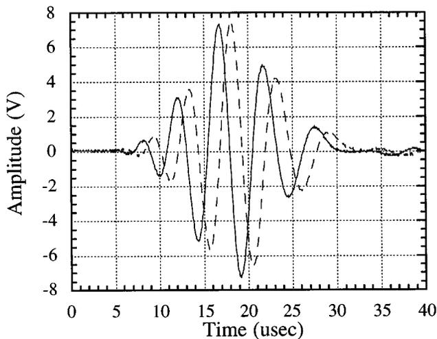
FIG. 5. Received waveforms for a 0.28-mm-thick (100) silicon plate in the [110] direction for two receiver locations 1.25 mm apart. The transmitter–receiver distance is 2.54 cm.
