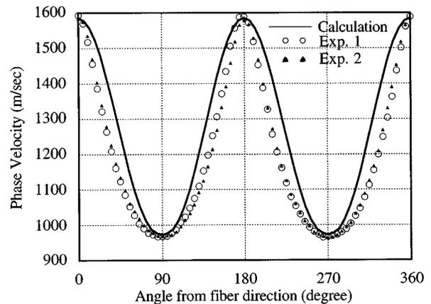
FIG. 10. Phase velocity variation of the A0 mode in a uniaxial composite plate of thickness 1.7 mm at 200 kHz. The circles and filled triangles are experimental data whereas the calculation is plotted as a solid line.
