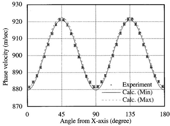
FIG. 8. Phase velocity variation of A0 mode in the same silicon sample in Fig. 4. The squares indicate experimental data with the error bars and the solid and dashed lines are the calculated extrema for anisotropic phase velocity.
