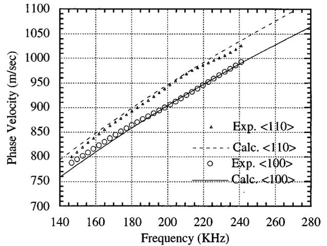
FIG. 9. Experimental and calculated dispersion curves for the silicon sample in two different propagation directions.
