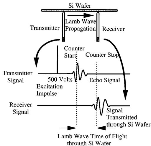
FIG. 3. Timing diagram for measuring time of flight of Lamb waves. The zero crossing of echo signal and the transmitted signal trigger the start and stop of the time counter.
