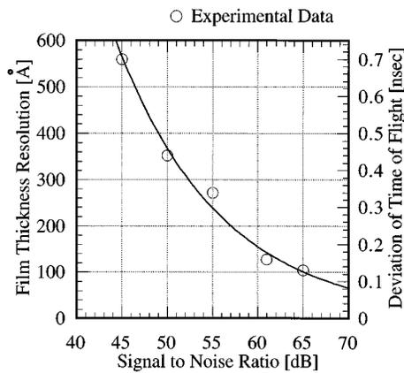
FIG. 6. Film thickness measurement accuracy as a function of SNR.
