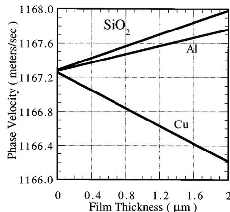
FIG. 1. Antisymmetric Lamb wave phase velocity vs thin film thickness. The frequency of operation is 200 kHz.
