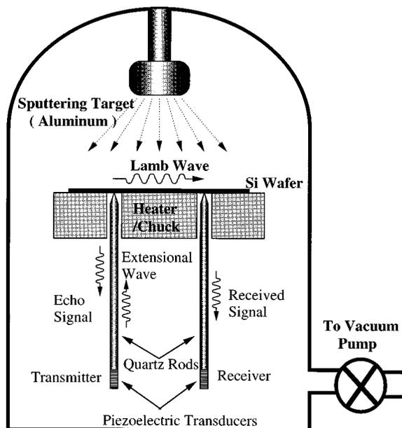
FIG. 2. *In situ* acoustic sensors implemented inside aluminum sputtering station.
