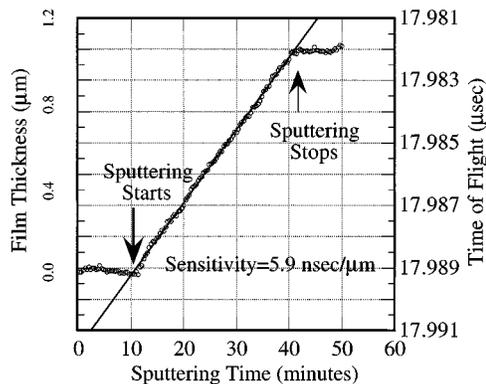
FIG. 5. *In situ* thin film thickness measurement. Time of flight decreases linearly during a 30 min run while  $1.2 \text{ }\mu\text{m}$  of Al film is grown.
