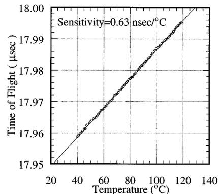
FIG. 4. Time of flight changes vs substrate temperature. The coefficient obtained is used to correct the time of flight data in the film thickness measurement.
