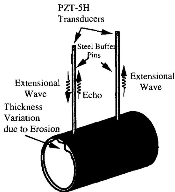
Figure 2. Experimental setup of pipe wall thickness measurement. Two PZT-5H transducer and steel buffer pin sets are used as the Lamb wave transmitter and receiver. The steel pipe under study has a diameter of 35cm and wall thickness around 10mm.
