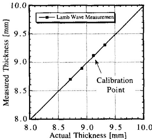
Figure 4. Calibration measurement is performed on a steel step wedge plate with thickness measured using a micrometer. With known distance between the transmitter and receiver pin tips, one point of the time of flight data is corrected for the electronic delay and fitted to the theoretical dispersion curve. Other thickness points fit the calculated curve within 1% error.
