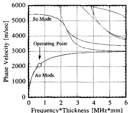
Figure 1. Theoretical calculation of the dispersion relation of steel plates.  $A_0$  mode is chosen in our experiment. The Lamb wave transducers are designed to have a frequency well below the cutoff frequency of higher order modes.
