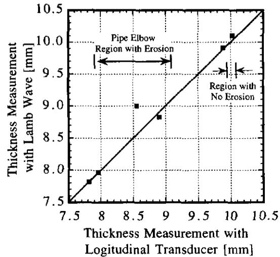
Figure 5. Thickness measurement performed on a section of steel pipe. Thickness variation measured with Lamb wave technique is plotted against the data obtained from a 10MHz longitudinal transducer.
