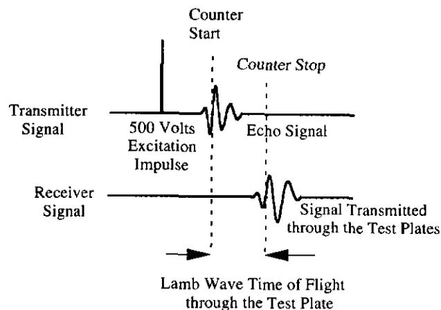
Figure 3. Timing Diagram for the time of flight measurement. The time delay from the echo signal and transmitted signal is measured. The effect of the two buffer pins is eliminated because the delays of acoustic signals in the transmitter and receiver buffer pins are identical.
