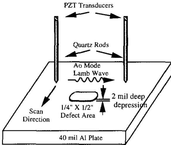
Figure 6. Imaging system for aircraft skin. A 2 mil (0.05mm) depression is milled into the aluminum plate to simulate a defect. 64 time of flight data point is take along each scan path. A total of 60 scans are taken at an interval of every  $3^\circ$ .
