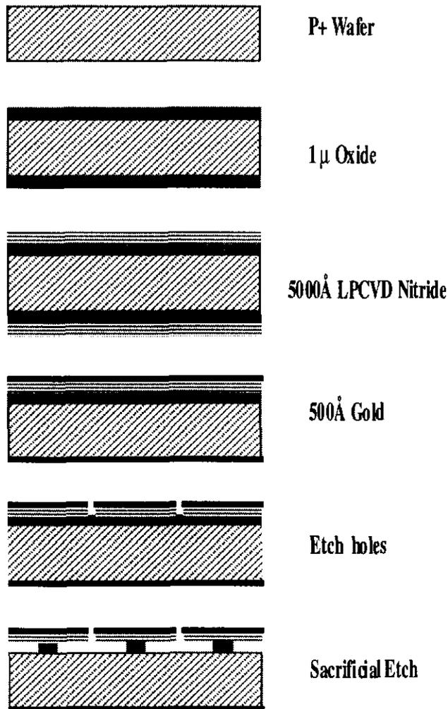
Figure 2: Fabrication sequence
