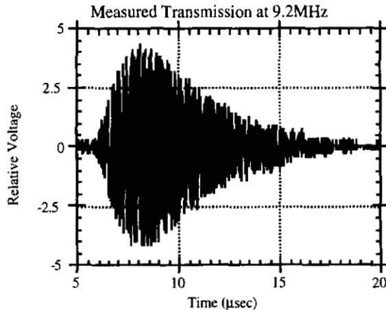
Figure 4a: Transmission at 9.2 MHz: Experiment
