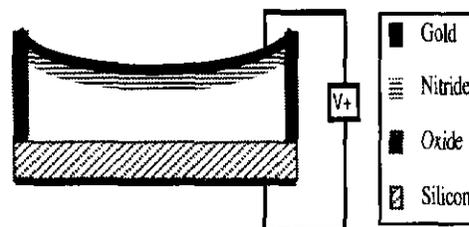
Figure 1: Schematic of one element of a MUT.
