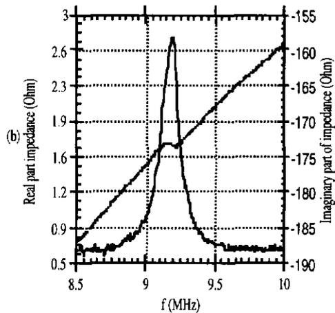
Figure 5: Impedance spectrum of 9.2 MHz device
