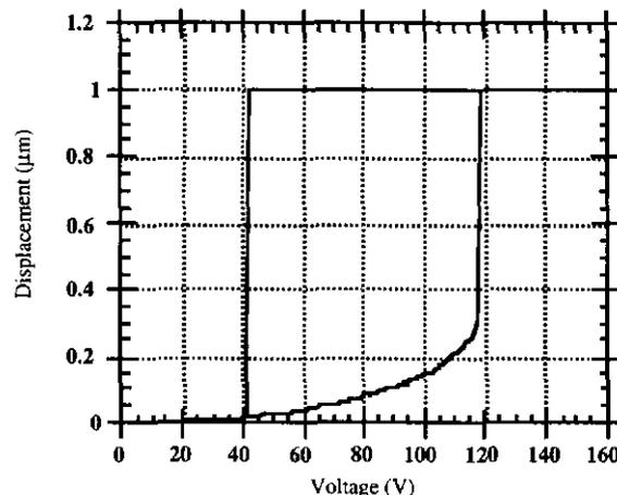
Figure 3: Collapse and hysteretic behavior of membrane.
