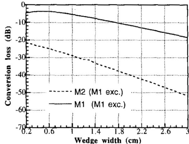
Figure 7. Conversion loss for two different Lamb wave modes showing the effect of side lobes in angular spectrum.
