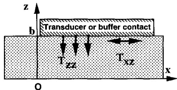
Figure 1. The plate geometry with coordinates. The plate is an unbounded anisotropic solid and has a thickness *b*.
