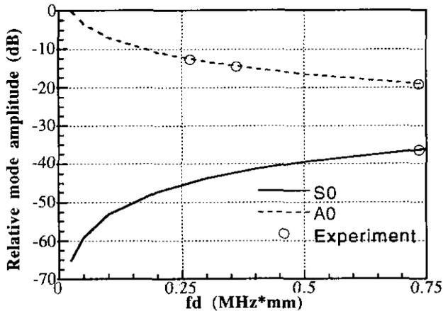
Figure 3. Relative Lamb wave amplitudes for A0 and S0 modes in (001) silicon for normal traction source on top surface. Circles indicate the experimental measurements.
