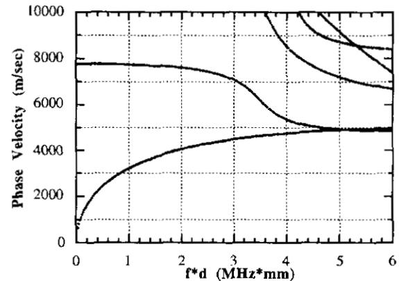
Figure 2. The Lamb wave dispersion curve for (001) silicon plate. Propagation is in  $\langle 100 \rangle$  direction.
