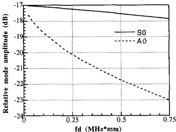
Figure 4. Relative mode amplitudes for A0 and S0 modes for tangential traction on top surface.
