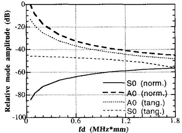
Figure 5. Relative mode amplitudes for A0 and S0 modes in steel plate normalized to A0 mode at  $fd=0.05$  MHz\*mm.
