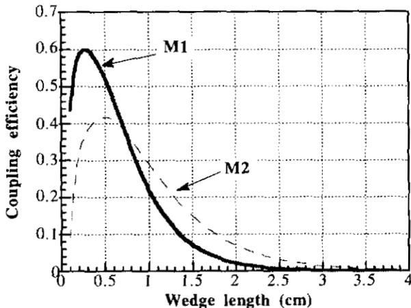
Figure 6. The excitation efficiency as a function of wedge width for two Lamb wave modes in aluminum plate in water,  $fd \approx 6 \text{ MHz*mm}$ .
