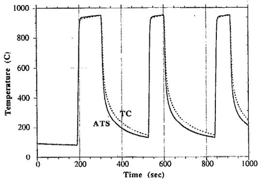
FIG. 5. Comparison of the acoustic temperature sensor (solid line) and reference thermocouple (dotted line) welded onto the center of the wafer.
