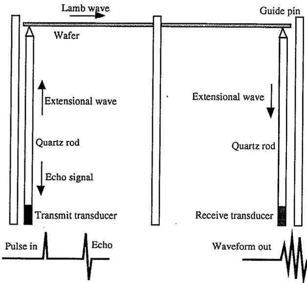
FIG. 1. Setup for measurement of silicon wafer temperature using acoustic techniques. The quartz support rod is used to transmit and receive acoustic waves. The guide pins prevent the wafer from falling off the pins during placement of the wafer in the reaction chamber.
