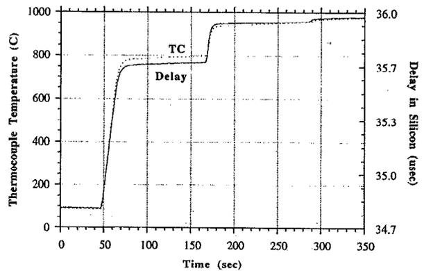
FIG. 3. Calibration run used to determine the Lamb wave velocity as a function of wafer temperature is steady state conditions.
