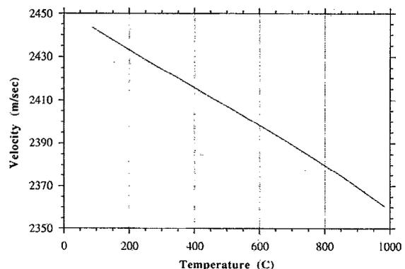
FIG. 4. Fourth-order polynomial model of the temperature dependent Lamb wave velocity given by  $T = 413\,870\,0 + 4479.1v - 1.289\,67v^2 - 5.8480 \times 10^{-5}v^3 + 4.9016 \times 10^{-8}v^4$ , where  $T$  is the temperature and  $v$  is the measured Lamb wave velocity.
