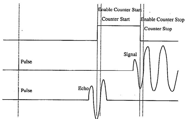
FIG. 2. Timing diagram for deriving time of flight of Lamb wave where pulse-echo signal is used to start the time delay counter and a specified zero crossing of the total time of flight signal is used to stop the counter.
