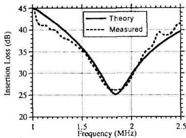
Figure 9. One way insertion loss (measured and theoretical) of the 100 µm period devices with 100 V bias voltage.
