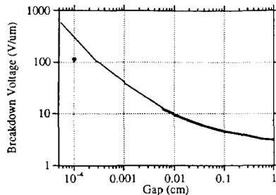
Figure 10. Breakdown field as a function of gap spacing.
