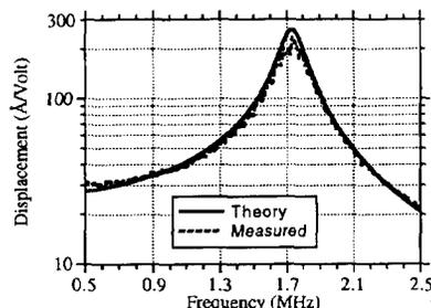
Figure 6 Measured and theoretical peak displacement for the 100  $\mu\text{m}$  period device with 100 V bias.
