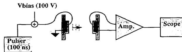
Figure 7. Schematic of acoustic measurement system.
