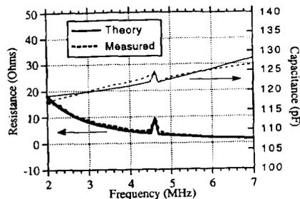
Figure 5 Measured and theoretical electrical impedance as a function of frequency for a 50  $\mu\text{m}$  period device.
