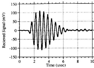
Figure 8 Received signal for experiment shown in Figure 7 with a transducer separation of 1 cm.
