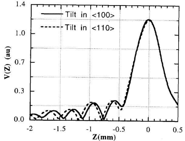
Figure 3. Calculated  $V(Z)$  curves for (100) silicon for two different tilt directions. Frequency is 48 MHz.
