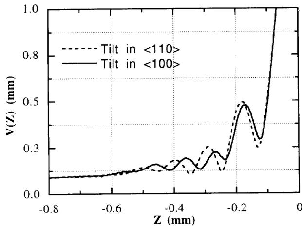
Figure 6. Measured tilted sample acoustic microscope  $V(Z)$  curves for (100) gallium arsenide sample with  $\theta_t=15^\circ$  in  $\langle 100 \rangle$  and  $\langle 110 \rangle$  directions.
