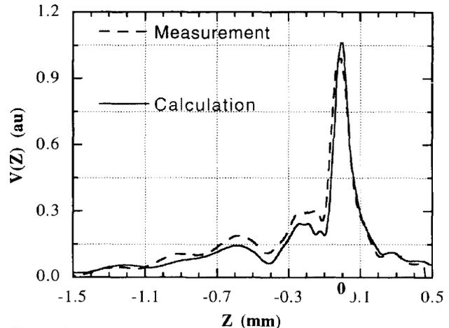
Figure 5. Calculated and measured  $V(Z)$  curves for (100) silicon sample with  $\theta_r = 10^\circ$  in  $\langle 100 \rangle$  direction. It should be noted that since the surface wave critical angle is much smaller than  $\theta_{max}$ , no anisotropy sensitivity is observed by changing the tilt direction.
