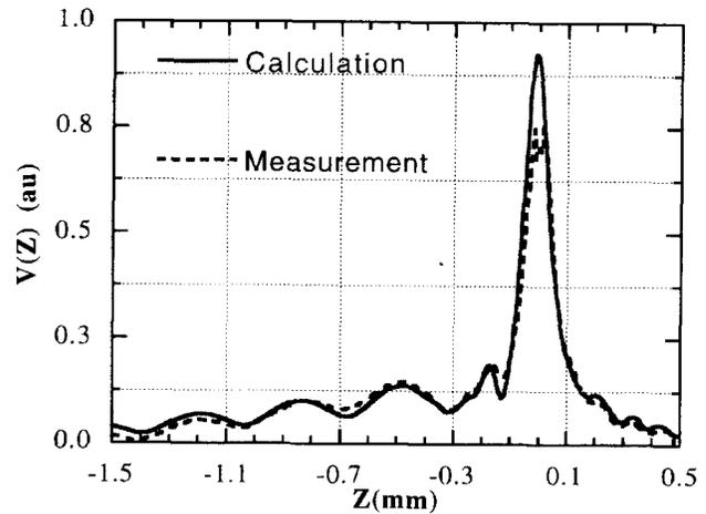
Figure 4. Calculated and measured  $V(Z)$  curves for (100) silicon sample with  $\theta_r = 5^\circ$  in  $\langle 100 \rangle$  direction.
