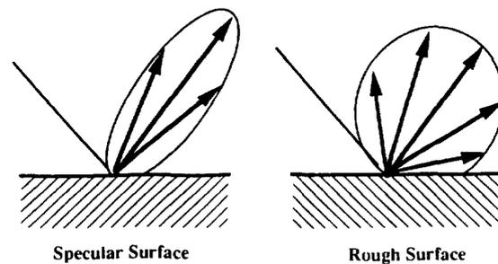
Fig. 6 Surfaces with different reflection properties can be simulated in the 3D simulator
