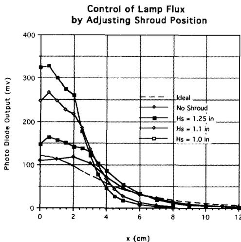
Fig. 4 Characterization and control of the light flux distribution for bulb with horizontal filament.
