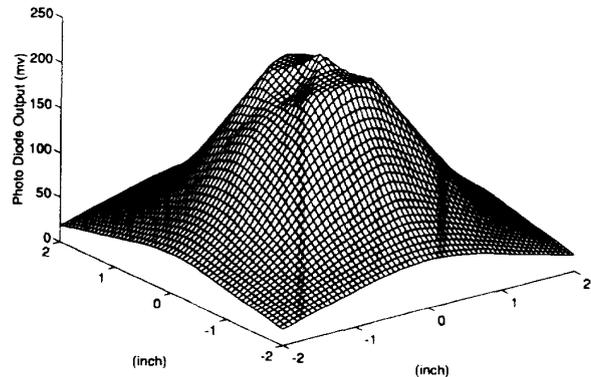
Fig. 5 A typical 3D light flux distribution from bulb with horizontal filament.
