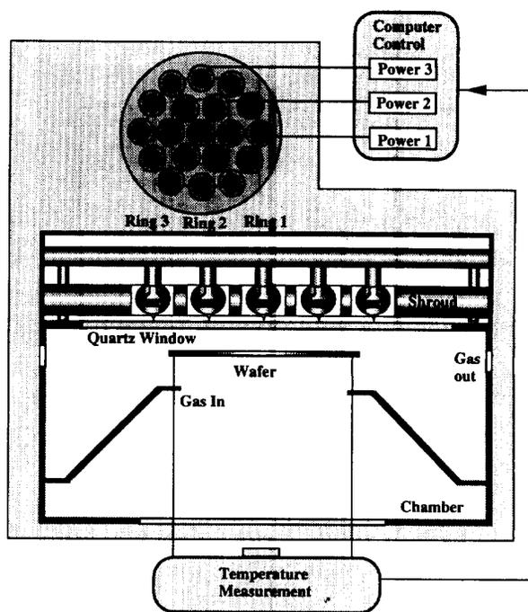
Fig. 1 A new RTP system with multi-variable and flexible lamp control. The power of each lamp ring is controlled independently and the position of shroud reflector can be adjusted to obtain the optimal lamp light flux distributions for various process conditions.
