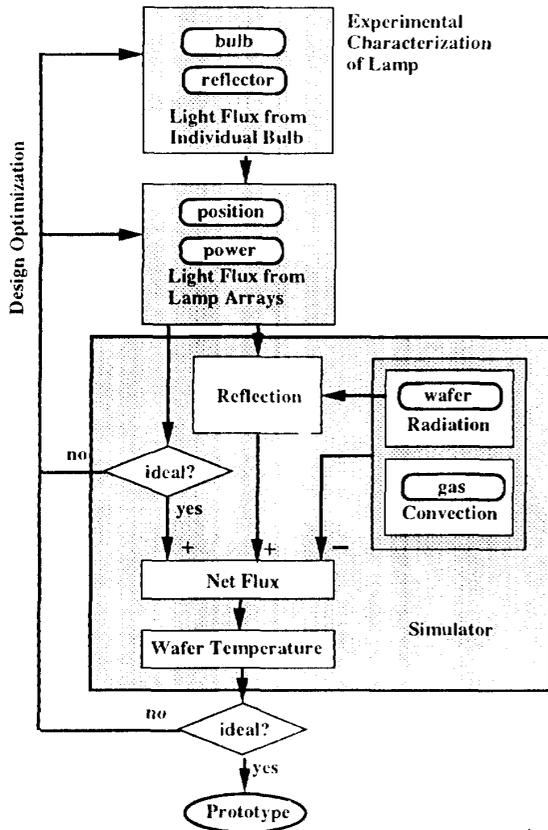
Fig. 2 RTP design methodology using 3D simulator
