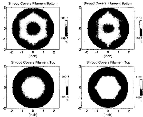
Fig. 8 Changing of shroud positions for different process temperatures ( 500 and 1100 °C).
