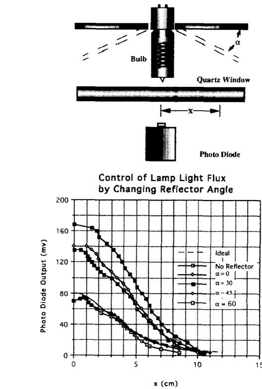
Fig. 3 Characterization and control of the light flux distribution for bulb with vertical filament.
