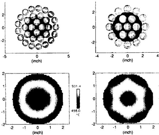
Fig. 7 Two different lamp array designs and their wafer temperature profiles.
