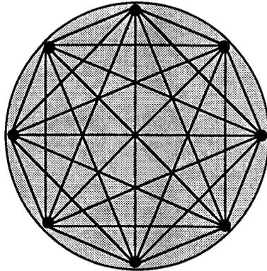
Fig. 10 Lamb wave paths for temperature mapping.
