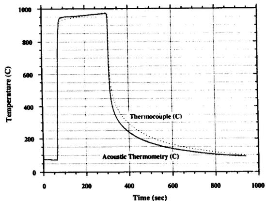
Fig. 8 Performance of the acoustic temperature sensor. Difference during the transients are due to the slower response of the thermocouple and the different positions of the thermocouple and acoustic path.
