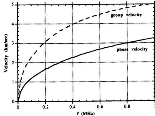
Fig. 2 Phase and group velocities of zeroth order Lamb wave as a function of frequency.
