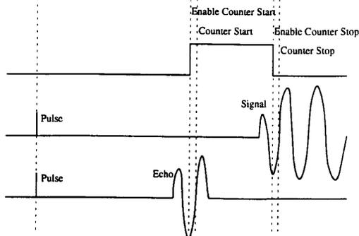
Fig. 4 Lamb wave time of flight measurement.
