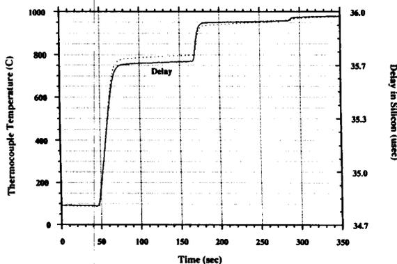
Fig. 6 Calibration run performed with a reference thermocouple.
