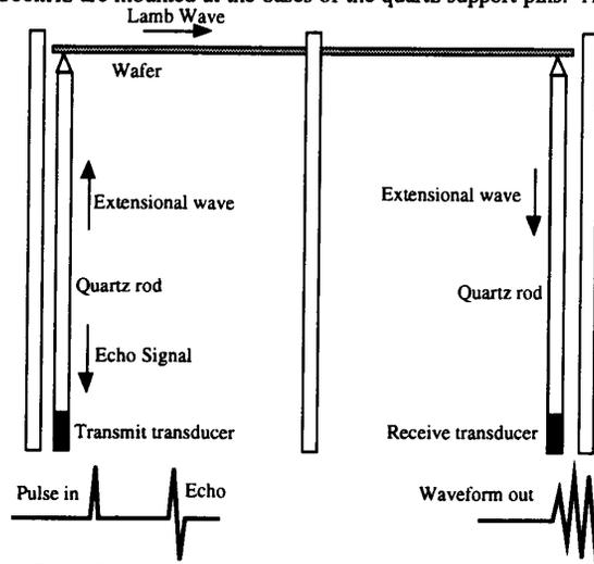
Fig. 3 Set-up of the acoustic temperature sensor.
