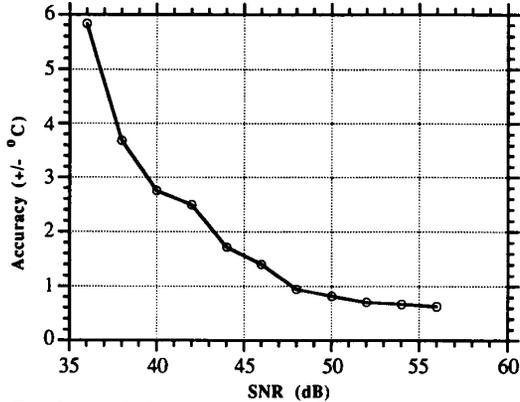
Fig. 9 Attainable accuracy as a function of the S/N of the measurement system
