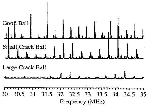
FIG. 2. Amplitude variation with crack size of surface-wave resonant modes. Samples are three  $\text{Si}_3\text{N}_4$  ceramic bearing balls. Diameter = 1/4 in.
