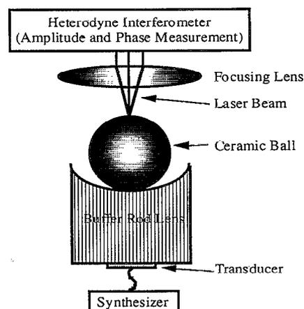
FIG. 1. Schematic of the one-point contact interferometric measurement technique.
