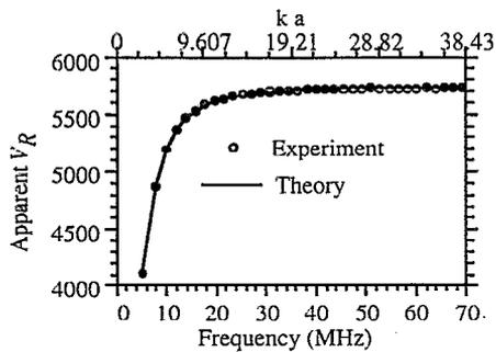
FIG. 4. Dispersion relation of surface waves on a sphere. Note that  $V_R$  used in the upper horizontal axis is the true Rayleigh wave velocity.
