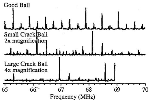
FIG. 3. Scrambling effect of surface-wave resonant modes in the high-frequency range. The interference of primary and secondary waves is apparent.
