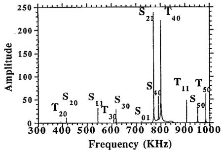
FIG. 2. Spectrum in amplitude for the fundamental modes of ball C.
