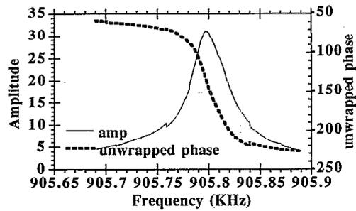
FIG. 3. Spectrum in both amplitude and phase for mode  $T_{12}$  of ball A. Curve fitting the phase information gives  $Q = 34\,799$ . One can see clearly the phase change near resonance.
