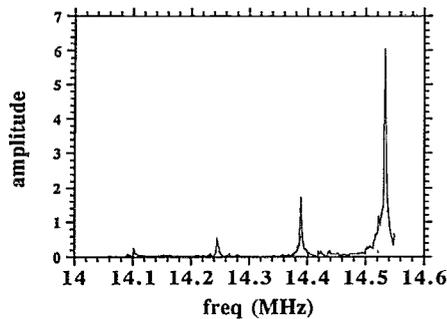
FIG. 4. Spectrum in amplitude for ball A around 14.25 MHz. The dominance of surface waves is evident.
