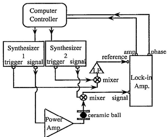
FIG. 1. Experimental setup for the resonant-sphere technique.
