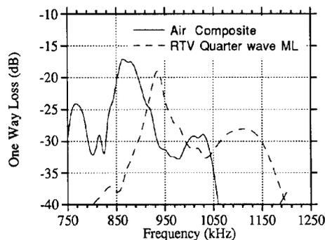
Fig. 6. Comparison of frequency response after 60 minutes of etching with reference PZT-RTV transducer.
