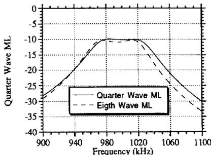
Fig. 4. Comparison of ideal performance of  $\lambda/4$  and  $\lambda/8$  designs for matching between PZT-5H and air at 1 MHz.
