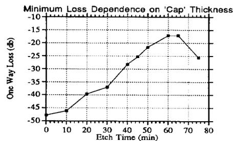
Fig. 5. Plot of transduction loss as a function etch time. ("cap" thickness starts at 56  $\mu\text{m}$  and thins a rate of 18  $\mu\text{m}/\text{hour}$ ).
