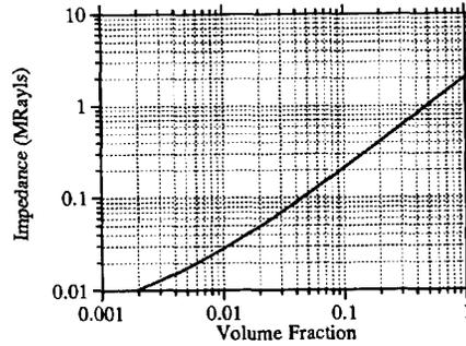
Fig. 2. Theoretical impedance of Kapton-air 1-3 composites.
