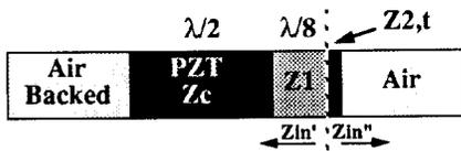
Fig. 3. Acoustic stack of  $\lambda/8$  design with high impedance "cap".
