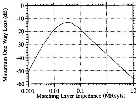
Fig. 1. One way transmission loss for a  $\lambda/4$  design matching between PZT-5H and air.
