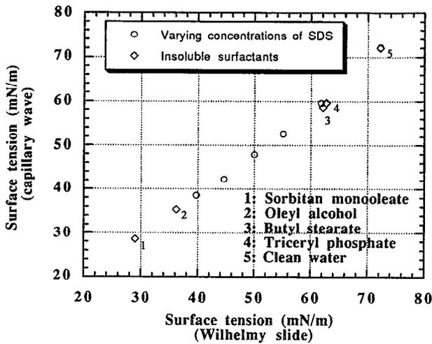
FIG. 3. Measured values of surface tension with different types of surfactants comparing the results of our technique with Wilhelmy plate technique.
