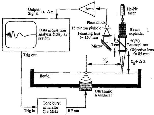
FIG. 1. Schematic of the capillary wave generation and detection system.
