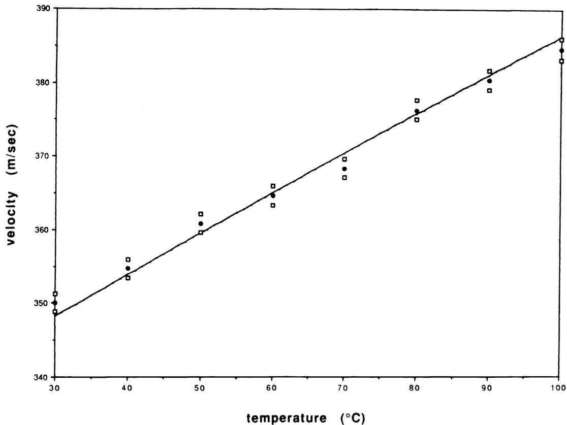
Fig. 4. Acoustic wave velocity in air as function of temperature.
