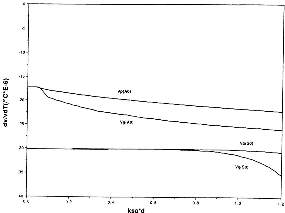
Fig. 1. Temperature dependence of plate mode phase and group velocities.
