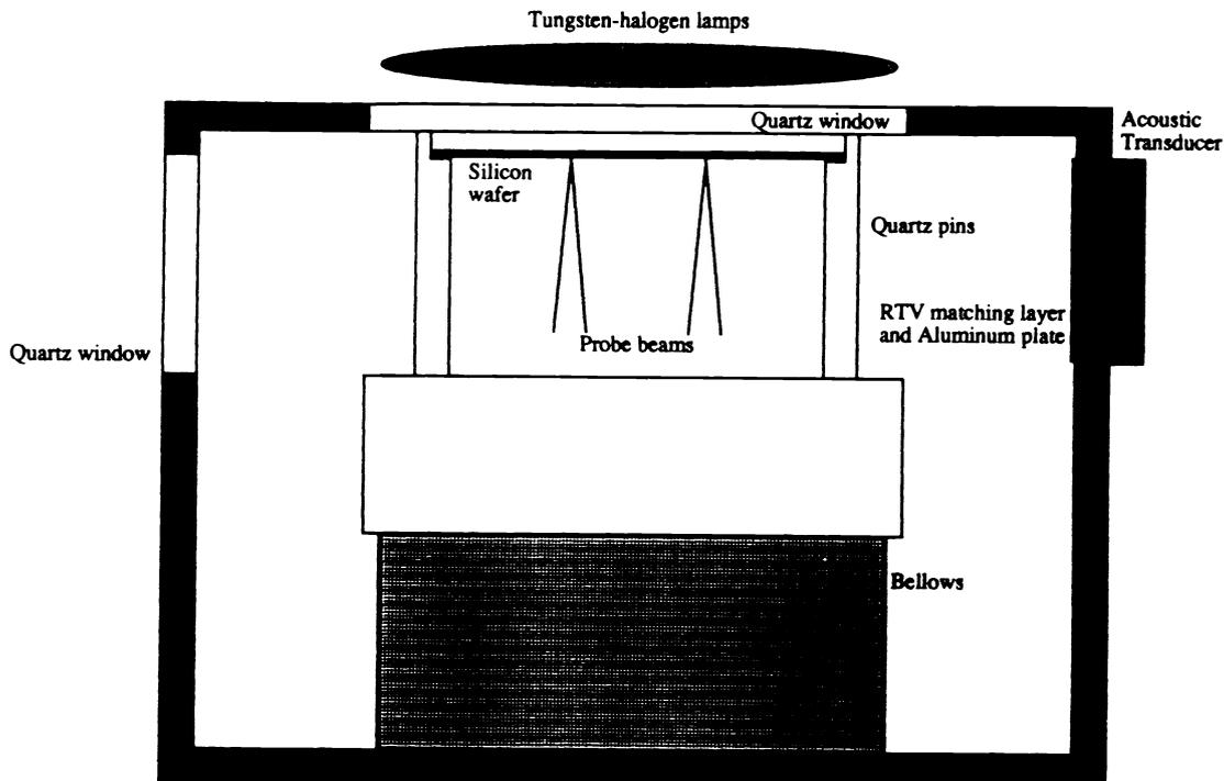
Fig. 3. Set-up for the temperature measurement of the layer of ambient directly above the silicon wafer.
