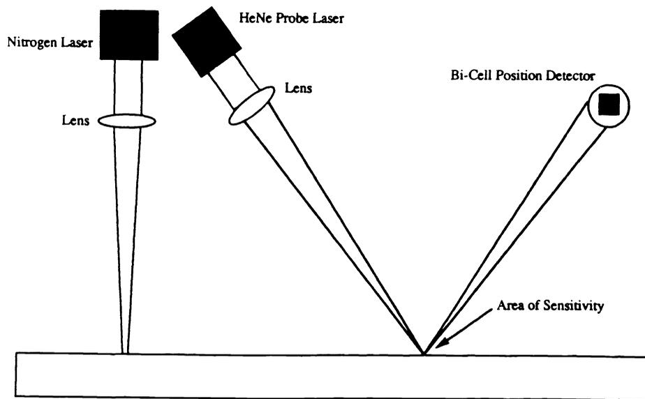
Fig. 2. Excitation and detection of acoustic waves.
