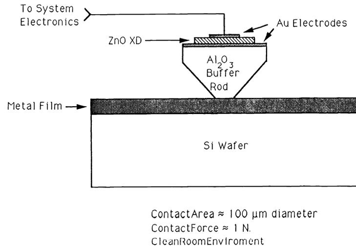
Fig. 1. Basic schematic diagram of acoustic TDR .
