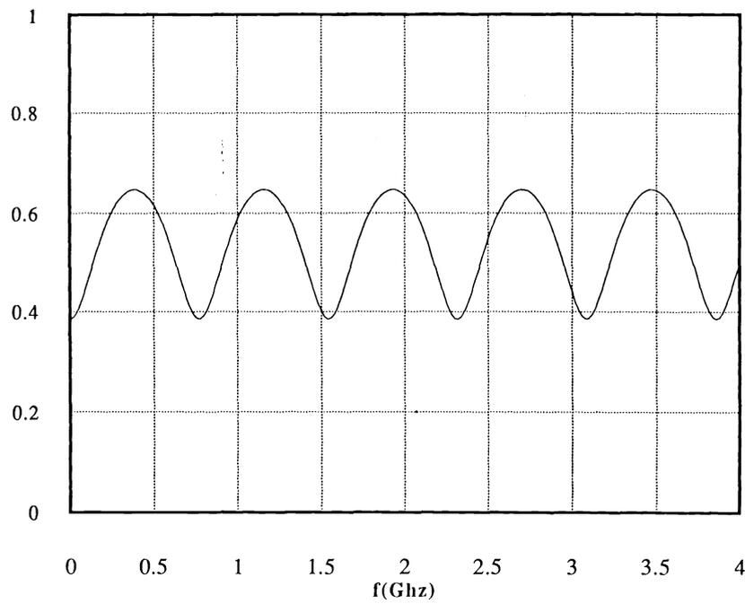
Fig. 2. Theoretical plot of reflection coefficient amplitude vs. frequency for  $2.1 \mu m$  gold film.
