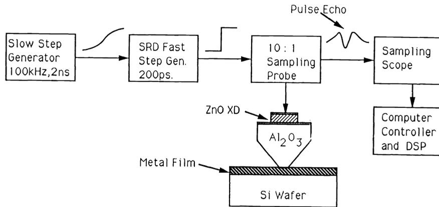
Fig. 4. Block diagram of acoustic TDR measurement system.
