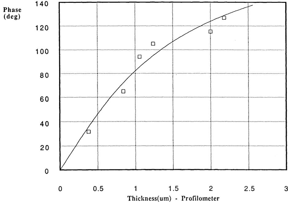
Fig. 3. Theoretical plot and experimental data of phase angle vs. film thickness for gold film. Acoustic propagation velocity  $V_0$  and the acoustic impedances of silicon and the metal film are required for an accurate film thickness measurement.
