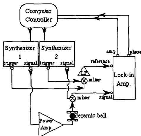
Fig. 1. Experimental set-up for the resonant sphere measurement.
