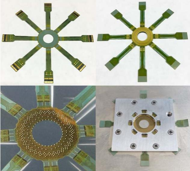
**Figure 4.** Optical image of flexible PCB. Back side (top left), bumped side (top right, bottom left) and flip chip bonding fixture (bottom right).
