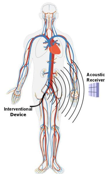
Fig. 1. Conceptual schematic of system for tracking interventional probes through thermoacoustic detection.
