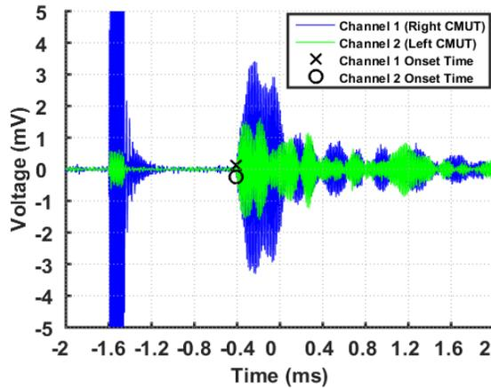
Fig. 4. Waveform showing onset of US signal used in time-of-flight calculations. Signal resulting from multipath reflection is seen after the initial onset of US signal.
