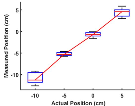
Fig. 6. Box and whisker plot for measured position vs. actual position in the horizontal dimension with  $N=100$  averages.
