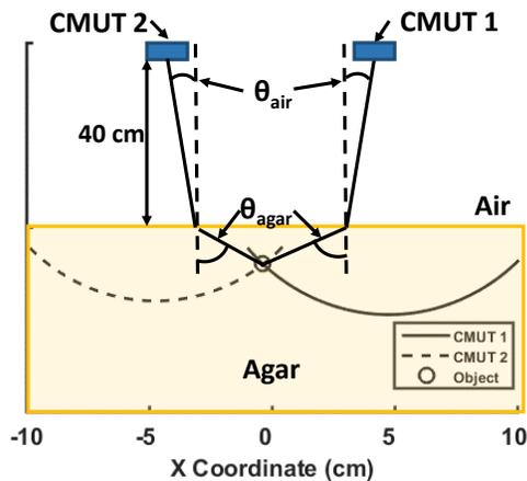
Fig. 5. Calculation of probe tip location with refraction.
