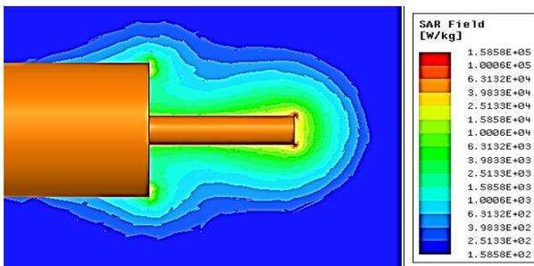
Fig. 2. Simulation of local SAR field magnitudes in log scale around exposed probe tip. Input power is 1 W and the probe is not matched to the source.
