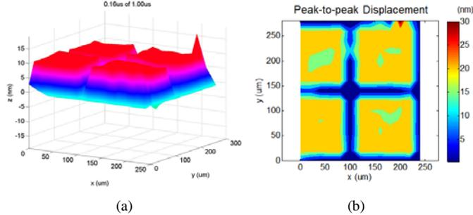
**Fig. 7.** Dynamic plate displacement measurement of a plain PCMUT: (a) a 3-D perspective view at the moment of the positive maximum peak and (b) a contour plot of a peak-to-peak displacement.
