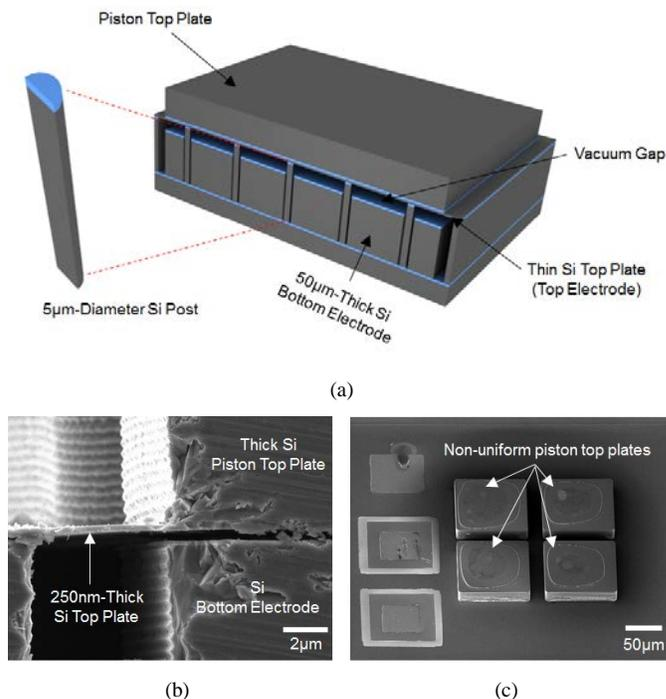
**Fig. 1.** (a) 3-D perspective view of a cross-sectional 2D PCMUT element. (b) Zoomed-in cross-sectional SEM image of the thin Si top plate. (c) 3-D perspective SEM image of second-generation PCMUT.
