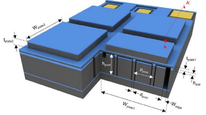
Fig. 3. 3-D perspective view of a single 2-D PCMUT element with the cross section of the fourth quadrant cell.
