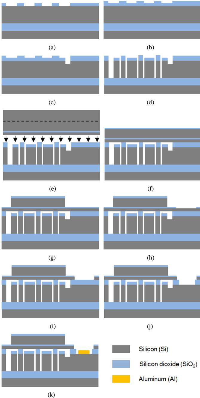
**Fig. 4.** Fabrication Process Flow. The cross-sectional view of A-A' line in Fig. 3. is shown, i.e. the first quadrant PCMUT cell with a bottom electrode pad.
