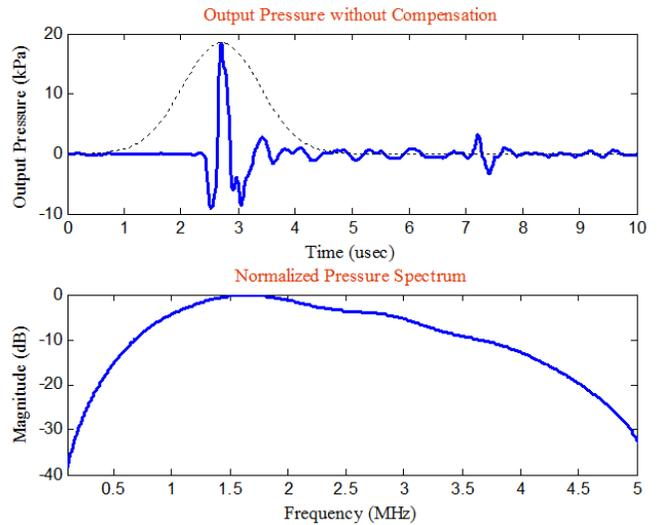
**Fig. 8.** Measured acoustic pressure of a truss PCMUT at 3.6 mm distance. (a) Transient pressure and (b) its frequency spectrum.
