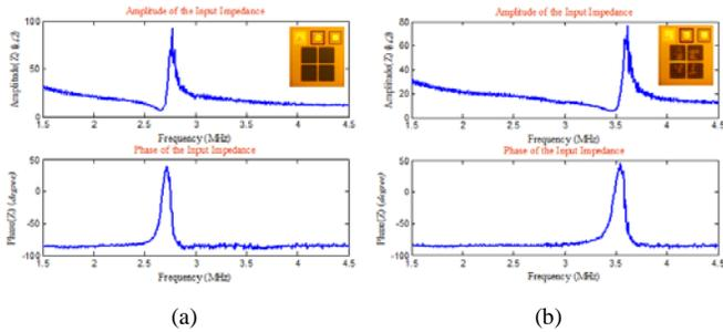
**Fig. 6.** Electrical input impedance measurement of PCMUTs with (a) a plain and (b) a truss piston top plates.
