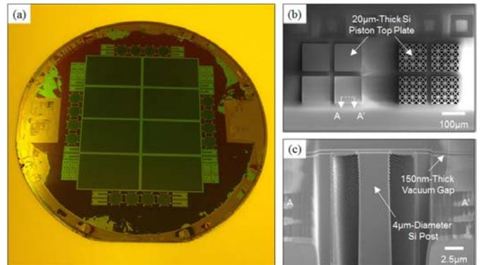
**Fig. 5.** (a) Optical photograph of a whole processed 4-inch wafer. (b) SEM image of two different types of 2D PCMUT elements. (c) Cross-sectional SEM image of A-A' line in Fig. 5(b).
