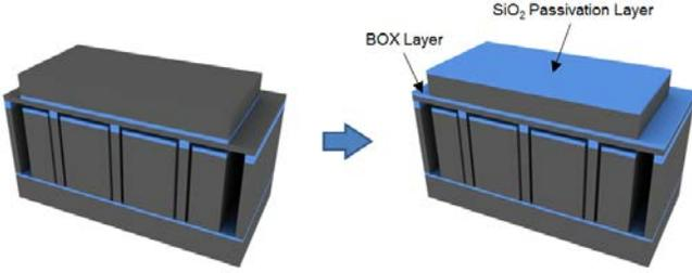
Fig. 2. 3-D perspective view of a single PCMUT element with the cross-sectional cut of the fourth quadrant cell.
