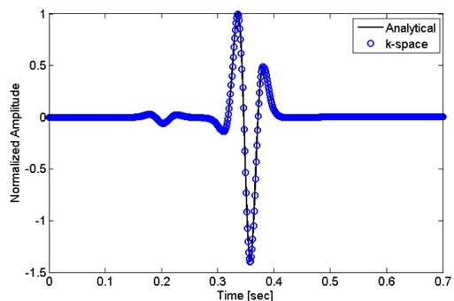
Fig. 2: The displacement profile along the axis of symmetry as a function time at 728.9m away from the source in a homogeneous three-dimensional transversely isotropic medium. Analytical solution (solid),  $k$ -space solution (circles).
