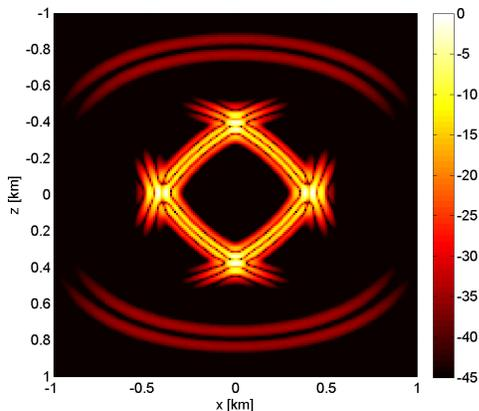
Fig. 1: Snapshot of the absolute value of the displacement field in a homogeneous three-dimensional transversely isotropic medium on the  $(y, z)$  plane at  $x = 0$ . The colormap is in the dB scale. Various wavetypes are in excellent agreement with the analytical ones [4], [5].
