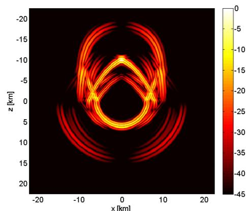
Fig. 3: Snapshot of the absolute value of the velocity field in the two-dimensional joint half-space problem. The colormap is in the dB scale. Various wavetypes are in excellent agreement with the ones of the previous studies [5], [6].
