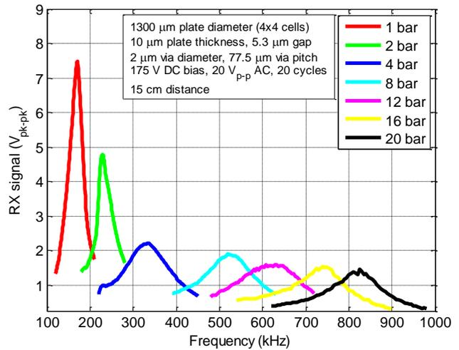
Fig. 5. Pitch catch measurement under varying ambient pressure
