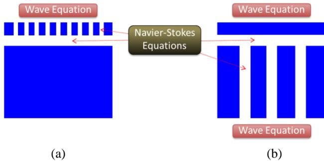
Fig. 1. Modeling fluid domains in a CMUT with vented cavities: (a) cavities vented through the plate, (b) cavities vented through the substrate
