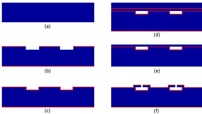
Single crystal Si Thermal oxide Aluminum
