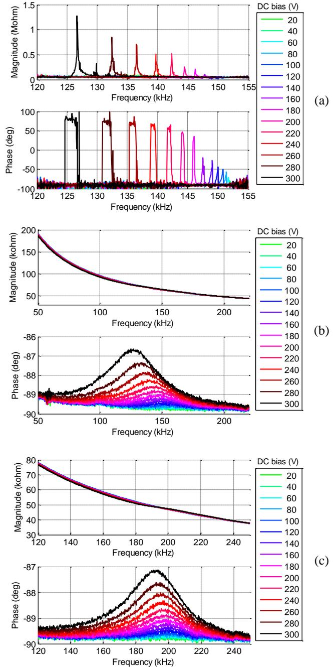
Fig. 3. Input impedance measurement: (a) measured in vacuum, (b) 1% vent area CMUT, measured in 1 atm, (c) 0.05% vent area CMUT, measured in 1 atm (Plate radius= 500  $\mu\text{m}$ , plate thickness = 10  $\mu\text{m}$ , gap height = 5.3  $\mu\text{m}$ )
