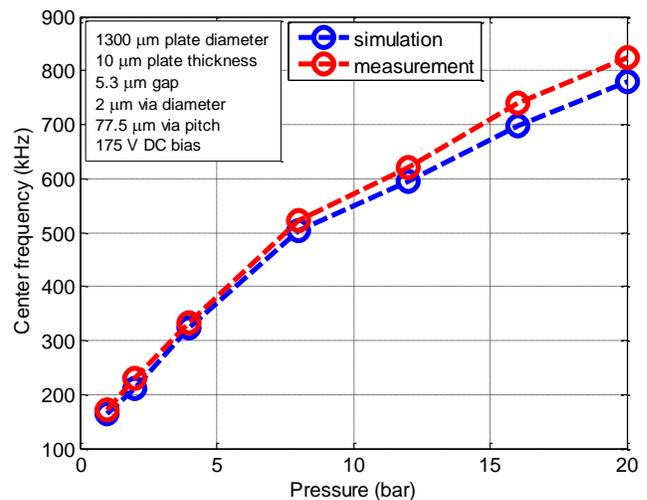
Fig. 6. Variation in resonant frequency with varying ambient pressure
