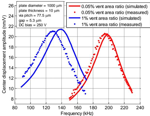
Fig. 4. Variation in squeeze film effect by varying size of vent holes
