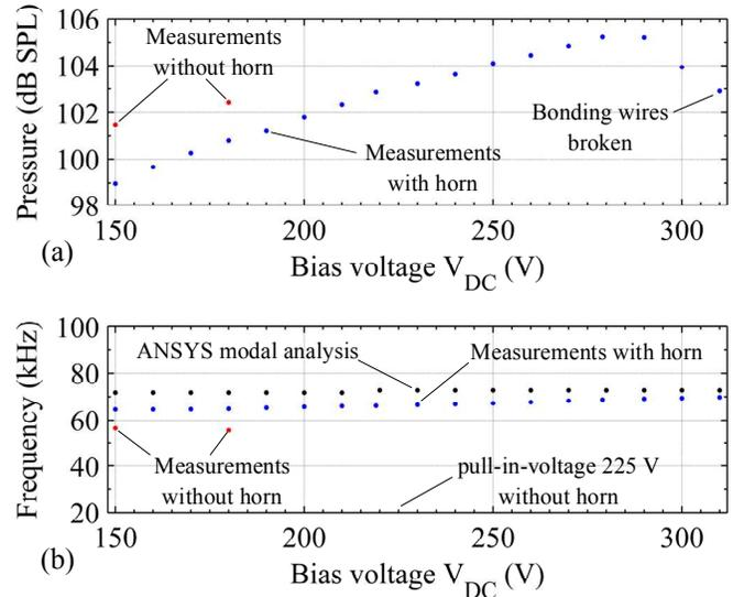
Fig. 4. Sound pressure levels (a) measured at a distance of 2.6 cm in front of the device with a calibrated microphone (B&K Type 4138, Skodsborgvej, Denmark) and a direct comparison of measured and calculated frequencies (b), all before and after gluing the horn at various d.c. bias voltages. The a.c. excitation signal was  $10V_{pp}$  and the pull-in voltage of the CMUT without horn is 225 V.
