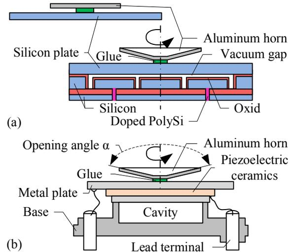
Fig. 1. Schematic of a circular single-cell air-coupled CMUT with an aluminum horn glued on top of the plate (a) and a sketch of a piezoelectric ultrasonic transducer (b), as specified in [8], [9]. For both devices the horn has an opening angle  $\alpha = 156^\circ$ . The top left insert in (a) shows a “horn” with an opening angle  $\alpha = 180^\circ$ , which could be fabricated with micromachining techniques [10].
