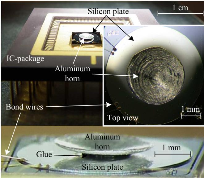
Fig. 3. Photographs of a 4-mm diameter single-cell air-coupled CMUT with an aluminum horn glued on top of the plate. The thickness of the horn is  $100\mu\text{m}$  and the diameter is 2.5 mm. The device is glued and wire-bonded to a standard IC-package for electrical connection.
