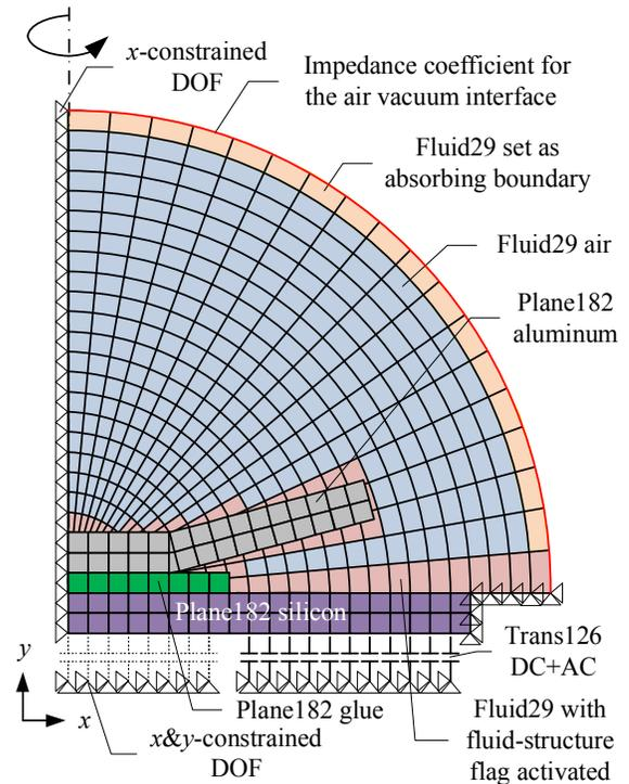
Fig. 2. Finite element model used for the calculation of the static, modal and harmonic response of a circular single-cell air-coupled CMUT with an aluminum horn glued on top of the plate.
