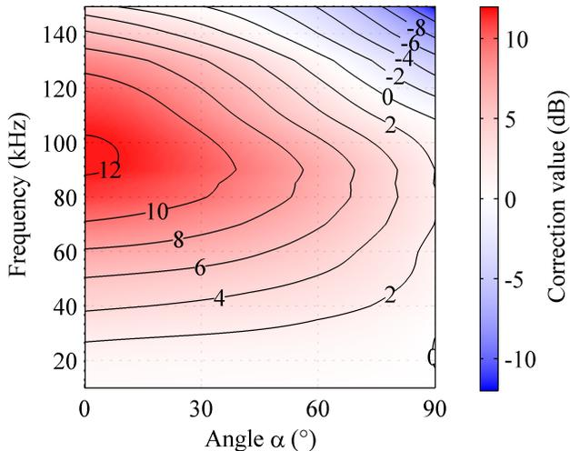
Fig. 3. Visualization of the total correction for free-field measurements. Shown is the ratio in dB between the measured pressure-response to free-field response for the B&K microphone (Type 4138).
