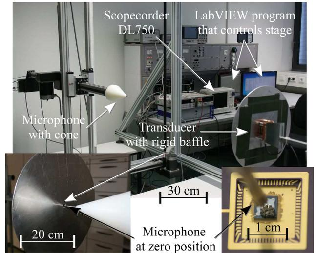
Fig. 2. Photograph of the measurement system, when configured to perform free-field measurements of a CMUT (bottom right) that operates in a rigid baffle (bottom left). The white cone has an angle of  $12^\circ$  and reduces standing waves between the stage and the rigid baffle.
