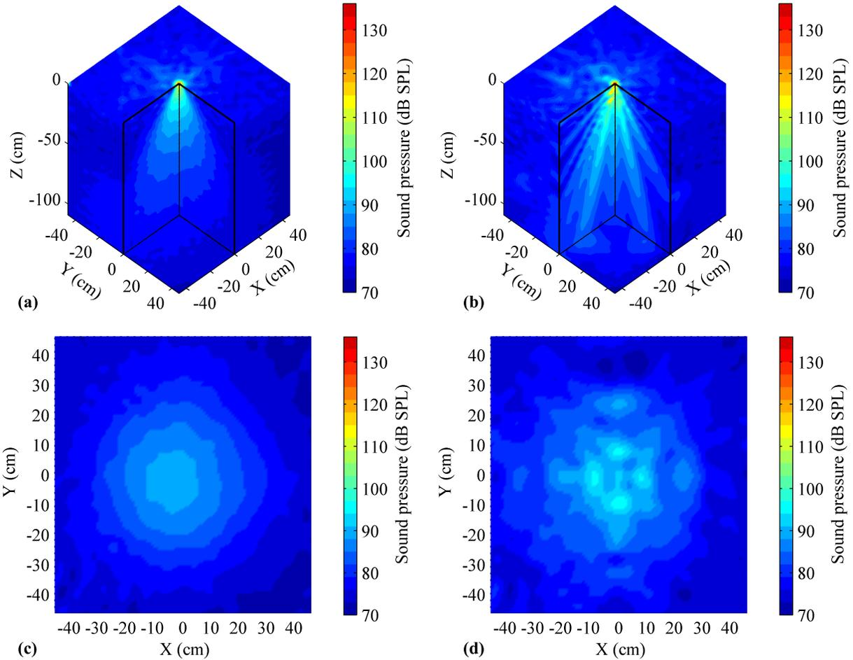
Fig. 4. Volumetric sound pressure fields (free-field, 3D with a cut-off section and 2D slices at a distance of 43 cm) produced by a CMUT in permanent contact mode mounted on an IC-package embedded in a rigid baffle. The two columns show two different measurement results corresponding to two operation modes for the CMUT. The right figure indicates a non-axial-symmetric velocity profile along the CMUT plate.
