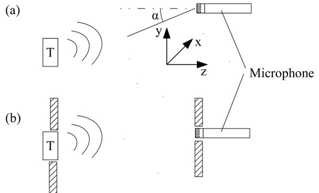
Fig. 1. Schematic of the volumetric measurement system. A microphone is used to sample a large volume in front of the transmitting transducer (T). The front face of the transmitting transducer and the microphone are kept in parallel. Depending on the acoustic boundary conditions, proper corrections about the microphone response must be applied for both (a) free-field measurements and (b) pressure response measurements with baffles.
