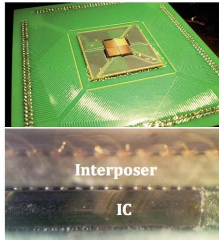
Figure 22.9.4: CMUT-Interposer-IC assembly wirebonded to a custom package (top). Side-view of the assembly showing the IC flip-chip bonded to the interposer (bottom).
