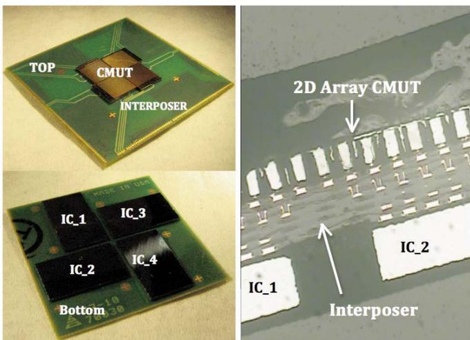
Figure 22.9.3: 3D stack (left) and cross-section (right) of CMUT-Interposer-IC assembly integrated using flip-chip bonding technology.
