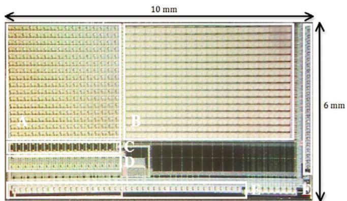
Figure 22.9.7: Die photo of IC. (A) Flip-chip pads, 256 pulsers and receivers. (B) Shift register and comparator array. (C) CMUT DC-bias pads. (D) 16 output buffers. (E) I/O and power pads.
