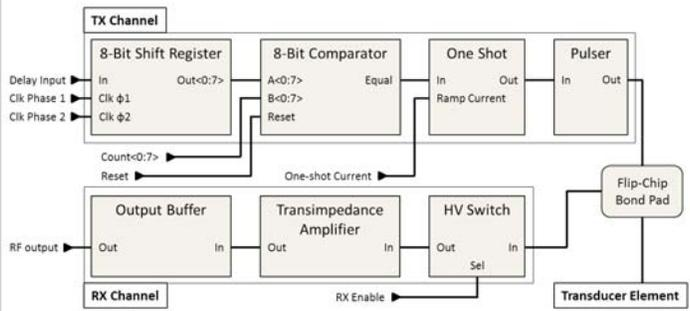
Figure 22.9.2: Block diagram of a single element of the IC.
