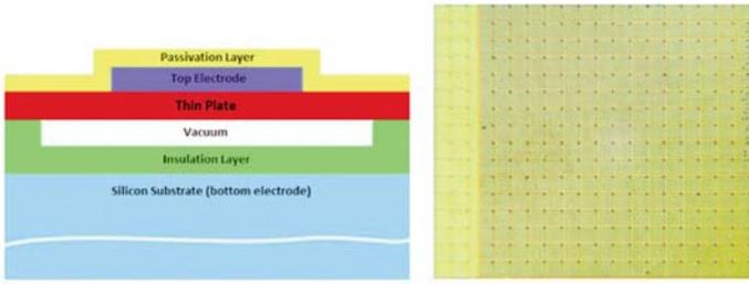
Figure 22.9.1: Basic CMUT cross-section (left) and 2-D 16x16 CMUT array (right).
