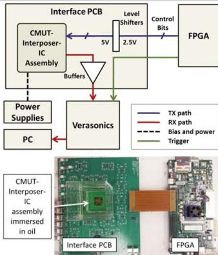
Figure 22.9.5: Block diagram of the experimental setup (top) and photograph of the interface PCB and the FPGA board (bottom).
