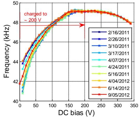
**Fig. 4:** The long-term measurement of the short circuit resonance of a pre-charged CMUT. The equivalent charged voltage stays nearly constant  $\sim 200 \text{ V}$  over a period of 19 months.
