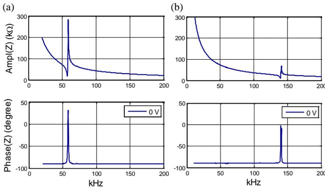
**Fig. 3:** The electrical impedance of CMUTs at zero-external-bias after charging: (a) A CMUT that is charged to  $\sim 82\%$  of the original pull-in voltage; (b) A CMUT charged to  $\sim 139\%$  of the original pull-in voltage.
