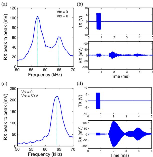
**Fig. 7:** The pitch catch measurement of a pair of pre-charged CMUTs. (a) and (b) show the results of no external bias applied to any of the CMUTs, while (c) and (d) show those of 50 V applied to the receiving device to match the frequencies of the pair. (a) and (c) are the peak to peak value of the receiving signal at different frequencies, while (b) and (d) are the time domain transmitting (TX) and receiving (RX) signals of the pitch-catch at  $\sim 64.5$  kHz.
