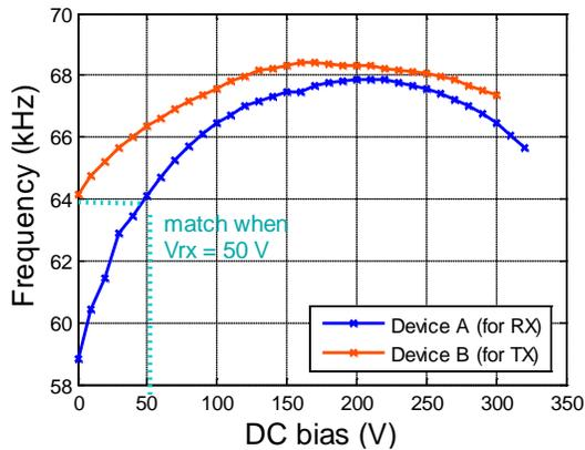
**Fig. 6:** The resonant frequencies of the pitch-catch pair at various external dc bias voltages. The two CMUTs operate at  $\sim 64$  kHz and  $\sim 59$  kHz, respectively, with no external bias voltage. Frequencies of the 2 devices match when a 50 V external bias voltage is applied to the receiving CMUT.
