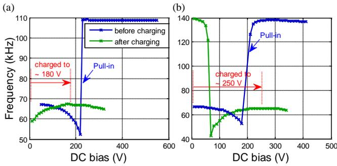
**Fig. 2:** The short circuit resonant frequency of two CMUTs before and after charging: (a) A CMUT that is charged to  $\sim 82\%$  of the original pull-in voltage; (b) A CMUT charged to  $\sim 139\%$  of the original pull-in voltage.
