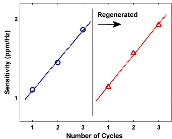
**Fig. 6.** Plot of volume sensitivity to CO<sub>2</sub> calculated from each cycle of exposing the sensor to 2-min CO<sub>2</sub> pulses from 0 ppm to 20,000 ppm in an increment of 4000 ppm, in N<sub>2</sub>. After three initial cycles, the polymer was regenerated and additional three consecutive cycles were applied.
