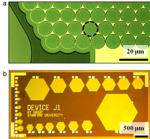
**Fig. 1.** Top-view optical pictures of (a) a section of a single sensor, showing multiple circular resonant structures connected in parallel to form a single device, and (b) a die showing an array of multiple sensors.
