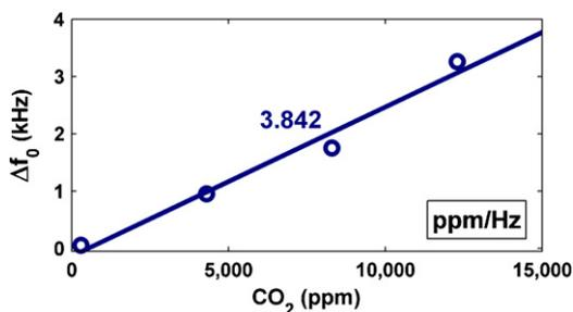
**Fig. 8.** Plot of maximum frequency shifts observed at different  $\text{CO}_2$  concentrations in air ( $\sim 45\% \text{RH}$ ).
