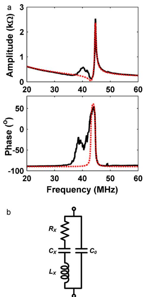
**Fig. 3.** (a) Plot of measured and fitted (dotted line) input impedance characteristics of the CMUT resonator biased at  $48\text{ V} \pm 50\text{ mV}_{\text{RMS}}$ , in air. (b) Schematic of 4-element van Dyke equivalent circuit model used to fit the input impedance data of the CMUT.
