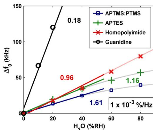
**Fig. 10.** Plot of maximum frequency shifts observed at different  $\text{H}_2\text{O}$  concentrations for four sensors and linear fits to estimate the volume sensitivities.
