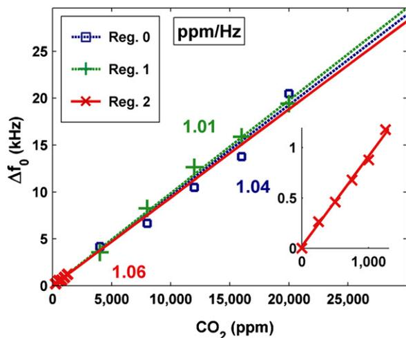
**Fig. 7.** Plot of maximum frequency shifts observed at different  $\text{CO}_2$  concentrations in  $\text{N}_2$  at the first cycle of each regeneration. The inset shows the maximum frequency shifts of the guanidine sensor exposed to a lower range of concentrations from 0 ppm to 1250 ppm demonstrating a distinguishable pulse as low as 250 ppm.
