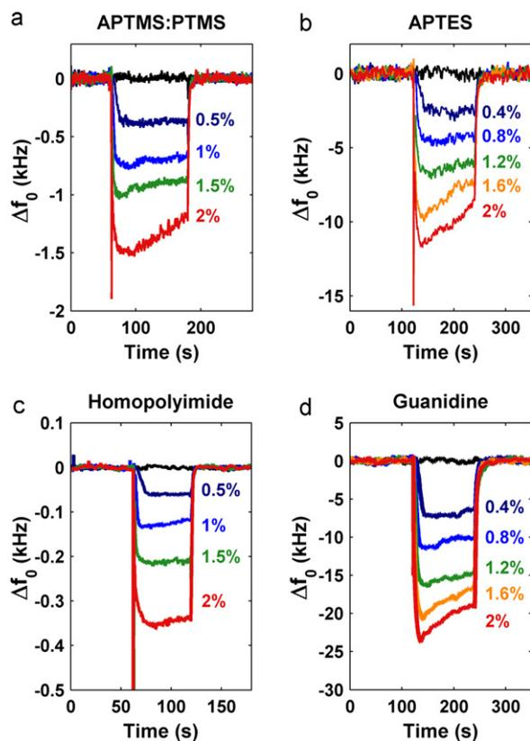
**Fig. 4.** Transient frequency shifts in response to various concentrations of CO<sub>2</sub> in N<sub>2</sub> of the CMUT sensors functionalized with (a) APTMS:PTMS, (b) APTES, (c) homopolyimides, and (d) guanidine. CO<sub>2</sub> starts to flow in at 60 s or 120 s and stops at 240 s or 360 s, respectively. The CO<sub>2</sub> concentrations are represented in % where 1% is equivalent to 10,000 ppm.
