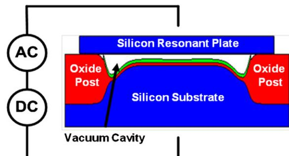
**Fig. 2.** Schematic cross-sectional view of a single circular CMUT resonator.
