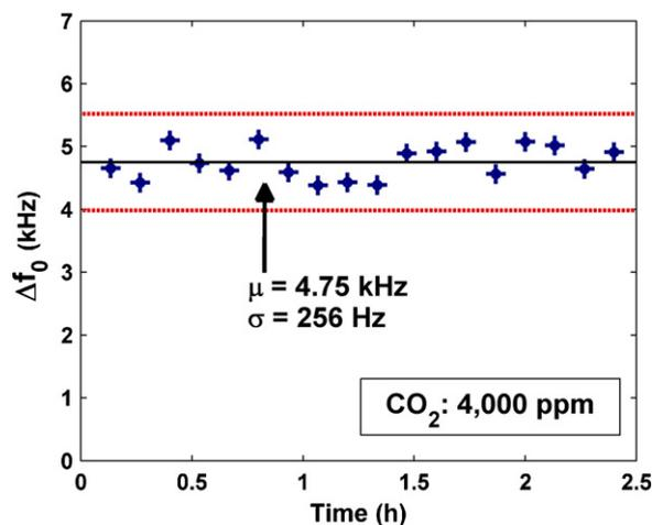
**Fig. 9.** Plot of maximum frequency shifts to 18 pulses of 4000 ppm  $\text{CO}_2$  concentration over 2.5 h showing the mean (black line) and  $\pm 3\sigma$  (dotted line) frequency shifts.
