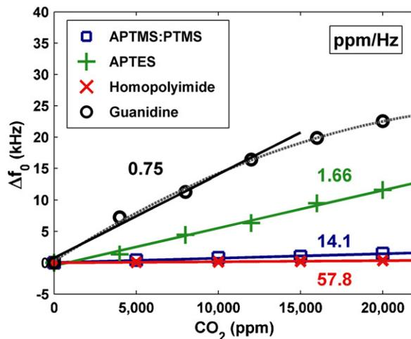
**Fig. 5.** Plot of maximum frequency shifts observed at different CO<sub>2</sub> concentrations in N<sub>2</sub> for four sensors. The numbers indicate the volume sensitivities in ppm/Hz which were estimated using the best-fit linear regression.
