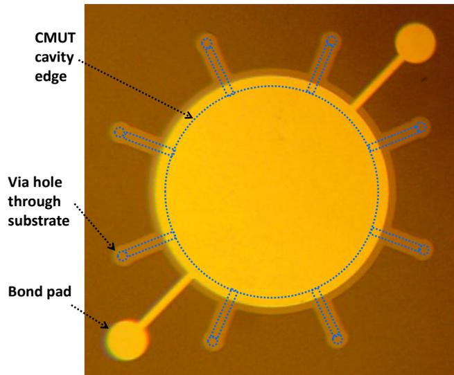
Fig. 3 Optical picture of a vented CMUT
