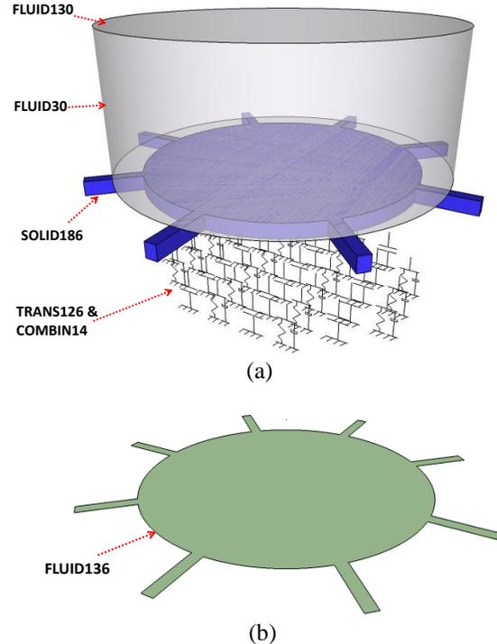
Fig. 2 Schematic of the ANSYS finite element models (a) 1<sup>st</sup> sub-model which includes the CMUT plate, fluid medium, transducers and spring-damper elements (b) 2<sup>nd</sup> sub-model which consists of the squeeze film elements overlaid on the bottom of the CMUT plate
