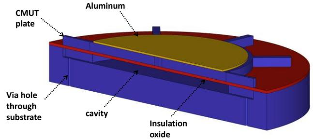
Fig. 1 3-D cross section schematic of vented CMUT structure
