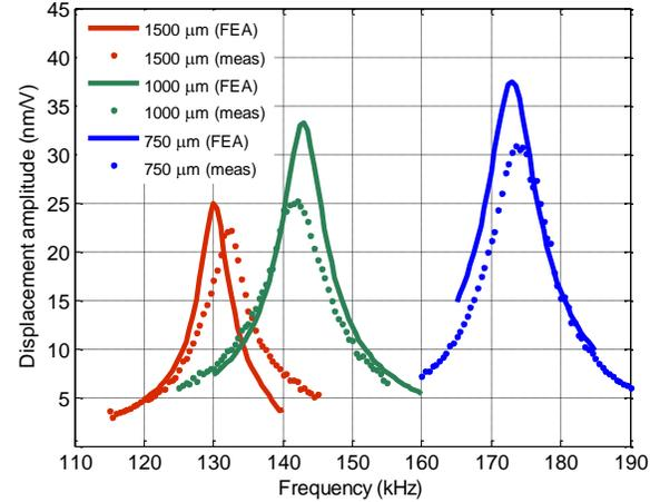
Fig. 4 vented CMUT amplitude measurements and comparison to FEA
