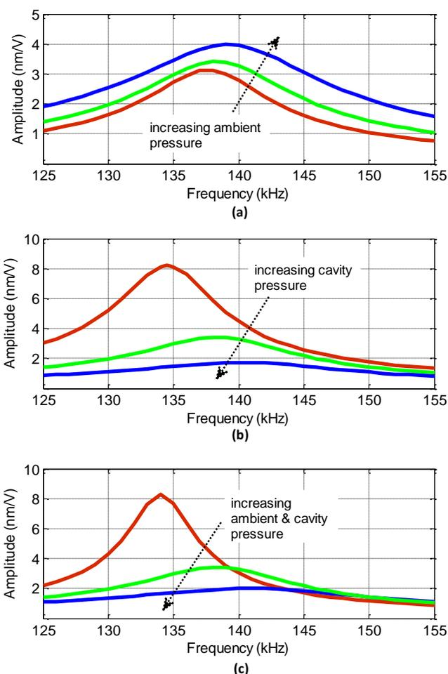
Fig. 5. Response of a vented CMUT with 20  $\mu\text{m}$  gap under varying ambient and cavity pressure (a) constant cavity pressure (2 atm) and increasing ambient pressure (1-3 atm) (b) constant ambient pressure (2 atm) and varying cavity pressure (1-3 atm) (c) ambient pressure = cavity pressure varying from 1 atm to 3 atm
