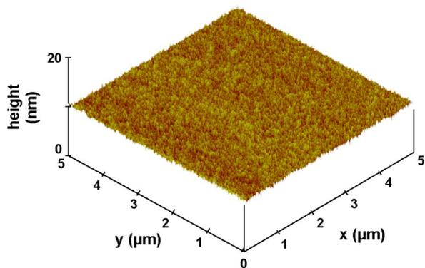
Fig. 5. AFM image of the flat area of the oxide post after the LOCOS process [Fig. 2(g)]. The measured surface roughness is  $2.36 \text{ \AA}_{\text{RMS}}$ .
