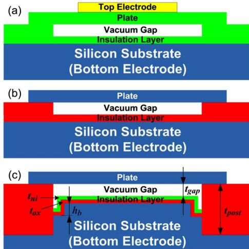
Fig. 1. Cross-sectional schematic of a CMUT based on (a) sacrificial nitride process, (b) conventional wafer bonding process, and (c) LOCOS/wafer-bonding process demonstrated in this paper.
