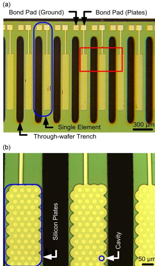
Fig. 8. Optical photographs of the fabricated CMUT. This particular device shown has a silicon plate with a thickness of  $0.5 \mu\text{m}$  and a cavity radius of  $9 \mu\text{m}$ . (a) Each element consists of 200 resonators (cells) and two bond pads to access the plate and the ground. Through-wafer trenches are located between the elements to reduce mechanical interference between the elements. (b) Zoomed-in picture of the red area in (a). The circular cavity is clearly visible.
