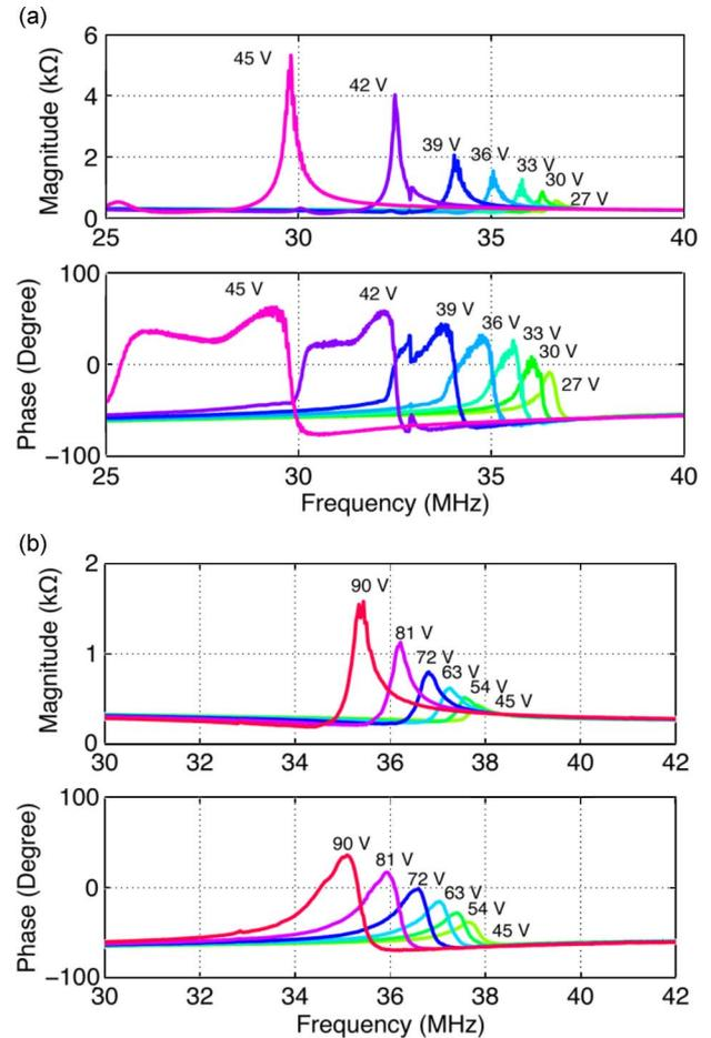
Fig. 9. Electrical input impedance of two devices in air. These devices have a plate radius of  $6 \mu\text{m}$  and a thickness of  $0.5 \mu\text{m}$  with (a) 40-nm gap and (b) 130-nm gap. A resonant frequency reduction due to the spring softening effect is clearly visible.
