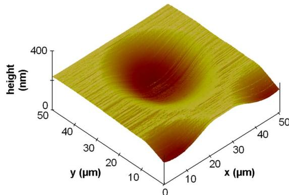
Fig. 6. AFM image of the silicon plate [Fig. 2(h)]. The static deflection due to atmospheric pressure proves that fusion bonding is successful because it maintains vacuum in the cavity beneath.
