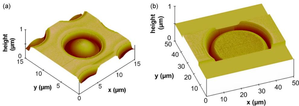
Fig. 4. AFM images of the cavity and the oxide post after the LOCOS process [Fig. 2(g)]. The measured step height between the oxide post and the silicon bump is (a) 39.8 and (b) 130 nm.
