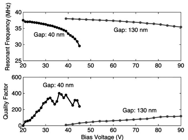
Fig. 10. Comparison of two devices with different gap heights. The resonant frequency and the quality factor are calculated from the measurements shown in Fig. 9.
