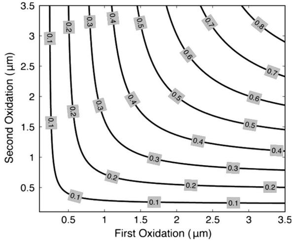
Fig. 3. Calculated height of the silicon bump [Fig. 2(d)] for different combinations of the first [Fig. 2(a)] and second oxidation [Fig. 2(c)] thicknesses.
