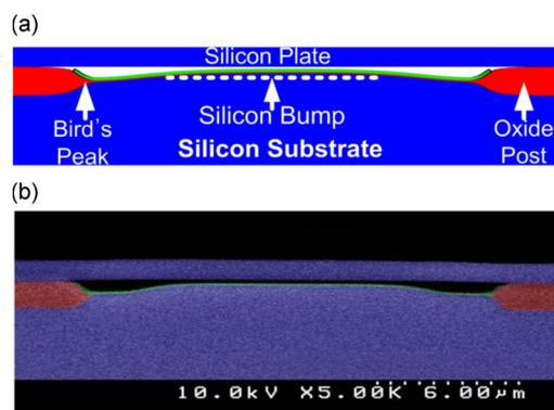
Fig. 7. Cross-sectional view of the CMUT cell by (a) TSUPREM simulation and (b) colored SEM of the fabricated device which has 130-nm gap. The color code is the same as in Fig. 2.
