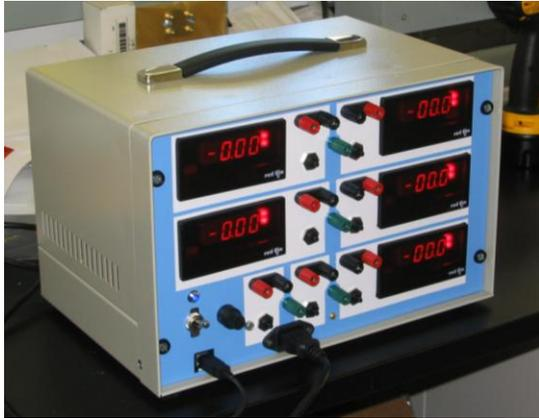
**Figure 8.** Power supply providing all necessary supplies to Ring catheter. Outputs can be monitored by a PC.
