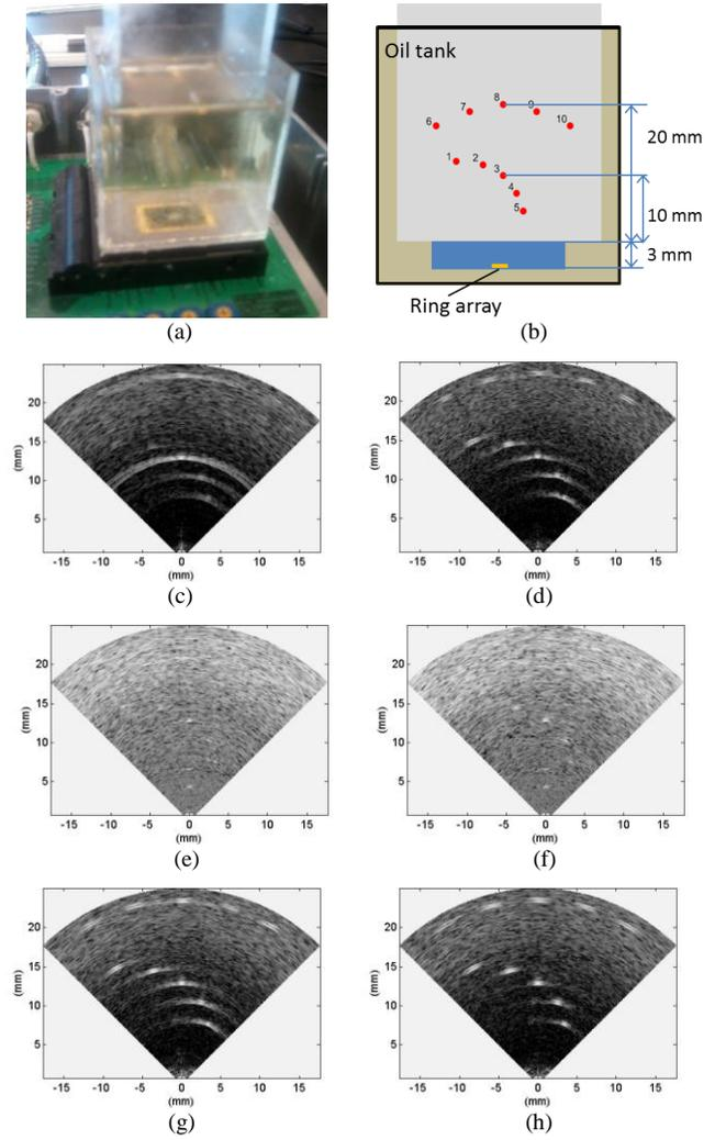
Figure 3. B-mode images of a phantom with 10 fishing wires, for six different imaging methods with a ring array, shown in 40-dB dynamic range. (a) Picture of the phantom in an oil tank (b) Location of each wire target (c) Flash (d) CPA (e) SPA (f) SPA-W (g) SPA-H (h) SPA-HW
