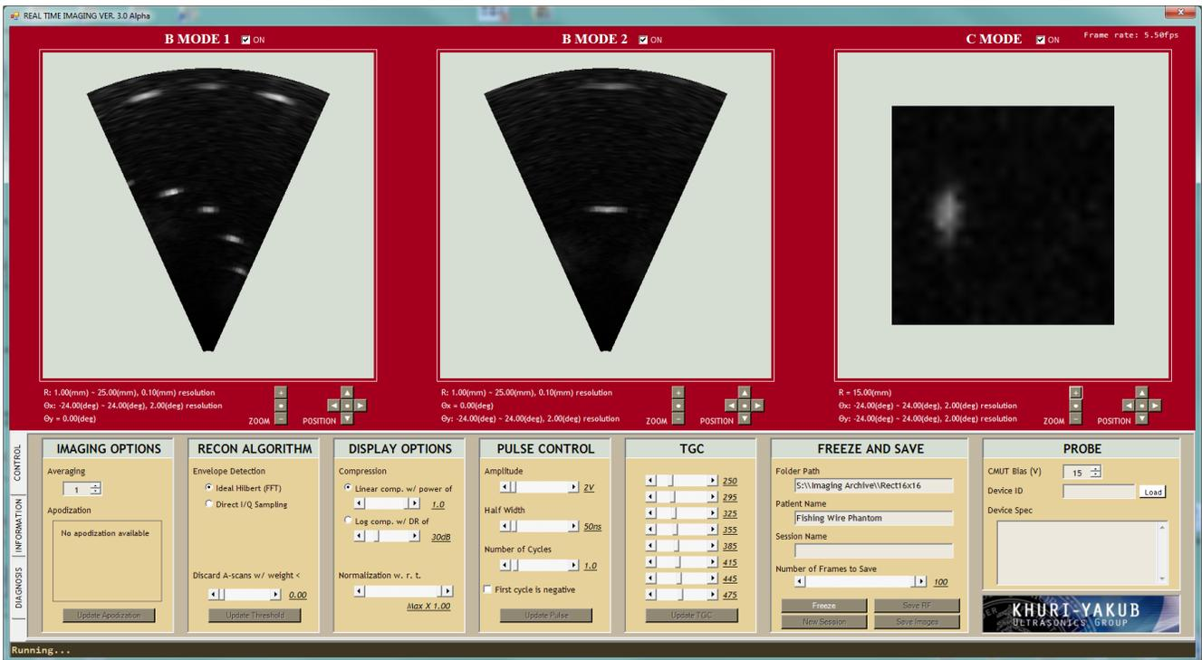
Figure 4. The custom software user interface, and real-time images of the fishing wire phantom, obtained with a  $16 \times 16$ -element rectangular array, using 625 focused beams. For transmit, we used unipolar pulses from the on-chip pulsers with 25-V amplitude and single cycle. The numbers in the Pulse Control panel are not used when the pulses are transmitted from the on-chip pulsers.
