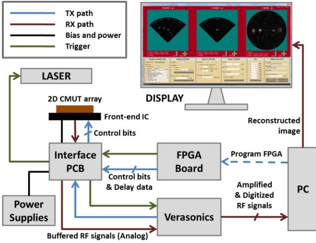
Figure 2. Top-level architecture of the system.
