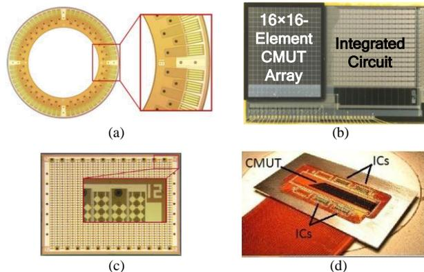
Figure 1. Various CMUT arrays with different geometry and electronics. (a) 64-element ring array (b) 16×16-element rectangular array (c) 24-element micro-linear array (d) 132-element linear array
