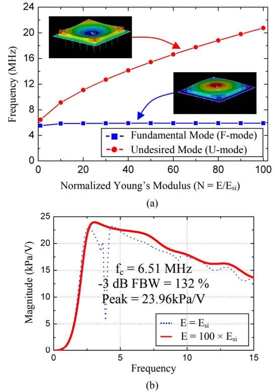
Figure 6. (a) Fundamental and undesired mode frequencies as a function of normalized Young's modulus of the top plate. (b) Average acoustic pressure spectrum showing the effect of large Young's modulus.
