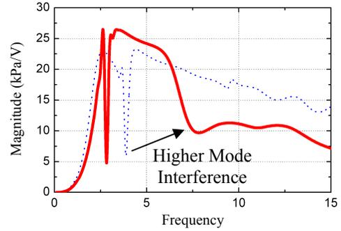
Figure 8. The average acoustic pressure spectrum of the second PCMUT design in table 2.
