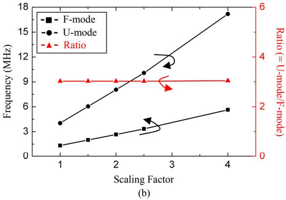
Figure 7. Fundamental and undesired mode frequencies as a function of (a) top plate thickness and (b) scaling factor
