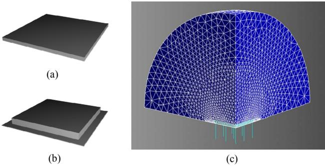
**Figure 2.** Schematic illustrations of two PCMUT top plate types: (a) type 1 and (b) type 2. (c) Schematic demonstration of the simplified 3-D FEA model of a PCMUT.
