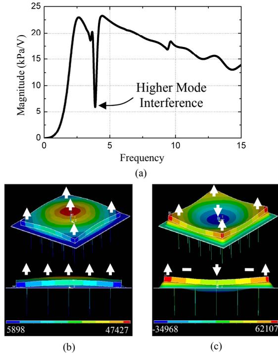
Figure 5. (a) The average acoustic pressure spectrum of the designed PCMUT structure. Modal analysis results of the designed PCMUT structure: (b) Fundamental mode and (c) first undesired higher mode.
