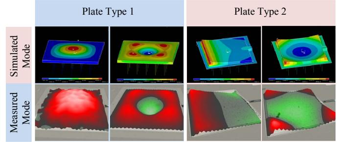
**Figure 3.** Simulated mode shapes vs. LDV measurements for plate types 1 and 2.
