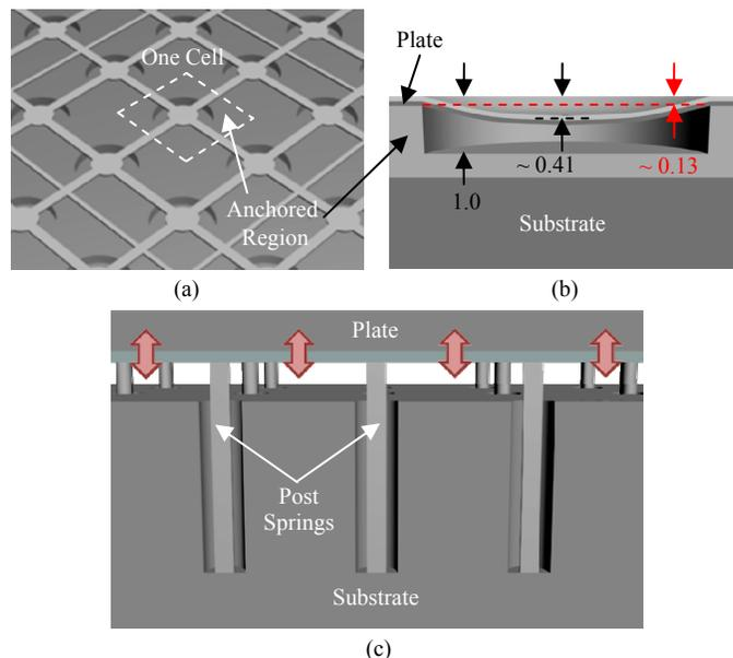
**Figure 1.** Schematic drawings of (a) a conventional CMUT array, (b) a CMUT cell, and (c) a PCMUT structure
