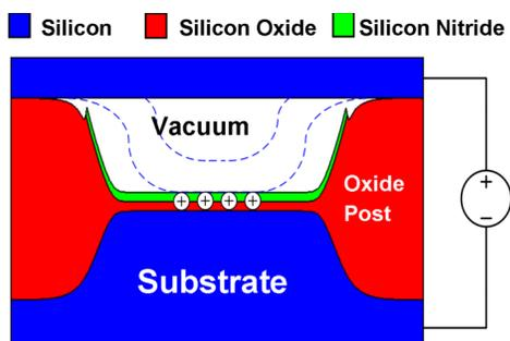
Figure 2. Cross-sectional schematic of one cell (not in scale). The thick oxide post layer ensures increased reliability with low parasitic capacitance during regular operation with external bias voltage, as well as during charge injection cycle. Blue dashed lines represent the plate during charging injection cycle.
