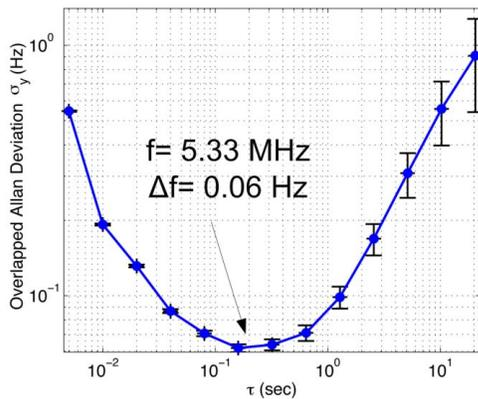
Figure 8. Overlapped Allan deviation calculated from the frequency counter with a gate time of 5 ms. The error bars indicate the 1-sigma confidence level.
