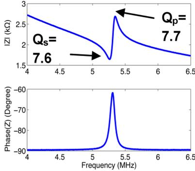
Figure 6. Measured input impedance characteristic of the zero-bias resonator after charge injection cycle, *i.e.* without external bias voltage. Quality factors,  $Q_s$  and  $Q_p$ , are calculated based on the magnitude of impedance and admittance, respectively.
