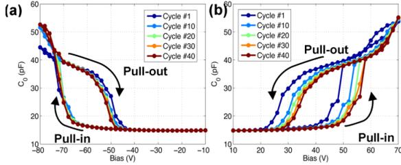
Figure 5. C-V measurement for complete pull-in/pull-out cycles with (a) negative and (b) positive bias voltages. Before the measurement, a 30-s pre-charging is applied by external bias voltages of (a) -80 V and (b) 70 V.
