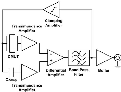
Figure 7. Circuit diagram of oscillator circuit.  $C_{comp}$  is selected to be same as device capacitance ( $C_0$ ). The topology of this circuit is based on a Pierce oscillator. An additional transimpedance amplifier with  $C_{comp}$  and a differential amplifier effectively compensate the effect of parasitic capacitance of the CMUT.
