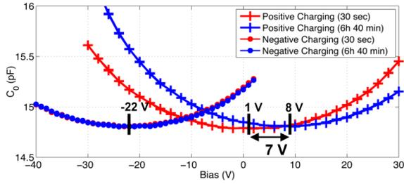
Figure 4. C-V measurement without pull-in cycle before and after the charging. The point of symmetry of each parabolic curve corresponds to the amount of built-in bias due to the charging in the insulation layers.
