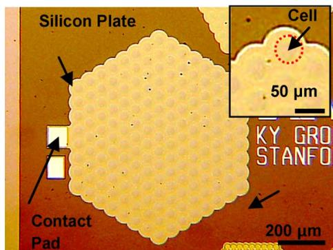
Figure 1. Photograph of the CMUT consisting of 169 cells, electrically connected in parallel. The vacuum cavities under the 500-nm-thick silicon plates are visible.
