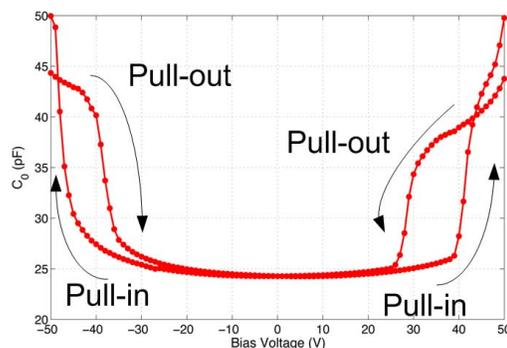
Figure 3. Exemplary C-V plot of a typical CMUT.
