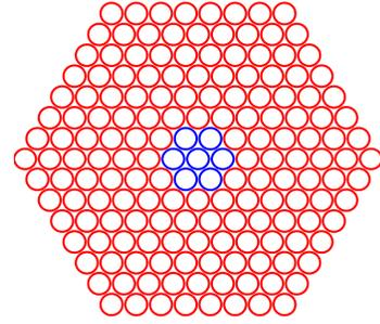
Figure 4. Diagram of cell locations in a hexagonal CMUT element. Blue circles represent a 7-cell CMUT, and blue and red circles together represent the 169-cell CMUT.
