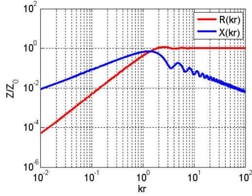
Figure 3. Real (R) and imaginary (X) part of acoustic impedance of single CMUT cell.
