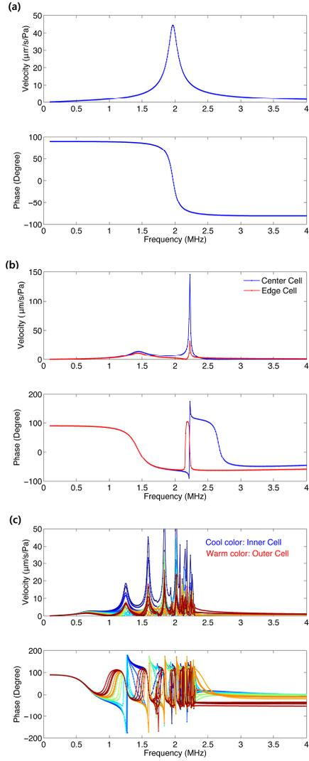
Figure 6. Frequency responses of average velocity of (a) 1-cell (b) 7-cell (c) 169-cell CMUT. In (c), the line color represents the location of the cell from the center of the element. The cells near the center are represented in blue color and the edge cells are in red color.
