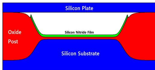
Figure 1. Schematic of cross section of a CMUT cell [8].
