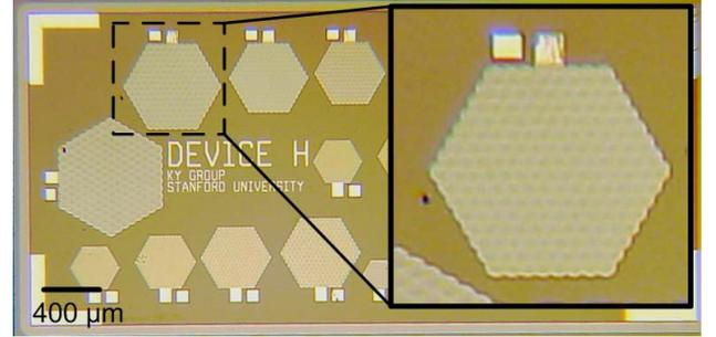
Figure 5. Optical picture of CMUT. The element in the zoomed picture is measured in this work. It has 169 cells in a hexagonal element configuration.
