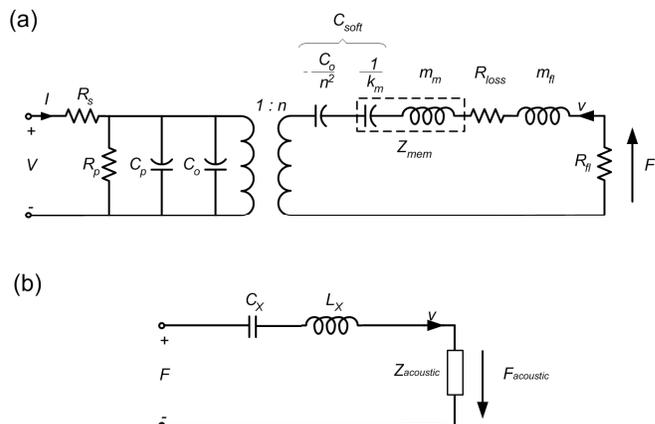
Figure 2. (a) Equivalent circuit of CMUT. All the components values are described in [5]. (b) Simplified equivalent circuit model.
