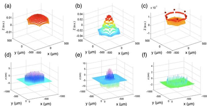
Figure 7. Calculated displacement pattern of 169 cells in the CMUT at (a) 0.67 MHz, (b) 1.3 MHz and (c) 4 MHz. Measurement of the displacement of the fabricated CMUT in immersion with an excitation frequency of (d) 0.7 MHz, (e) 1.26 MHz and (f) 4 MHz. The calculation results match well with the displacement measurement.
