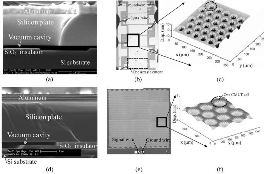
Fig. 3. Imaging CMUT pictures of the (a) SEM cross-sectional view of a cell, (b) six elements of one array with wire bonding, and (c) CMUT cells with plate deflection under dc bias of 80% of pull-in voltage measured by a white light interferometer. Similarly, HIFU CMUT pictures are shown in (d)–(f).
