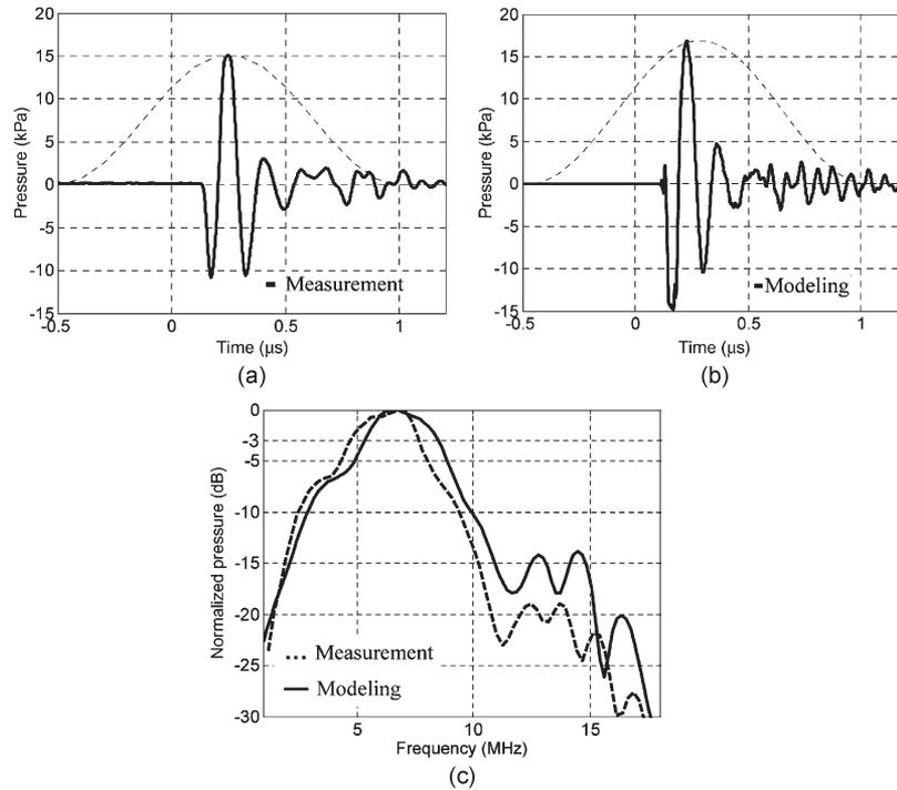
Fig. 11. Comparison between the (a) measurements and the (b) results from the viscoelastic model in the time domain, and (c) those in the frequency domain for the HIFU device with a CMUT cell radius of 50  $\mu\text{m}$  with 150  $\mu\text{m}$  of GE RTV 615 coating. The data was retrieved from the plate-PDMS interface.
