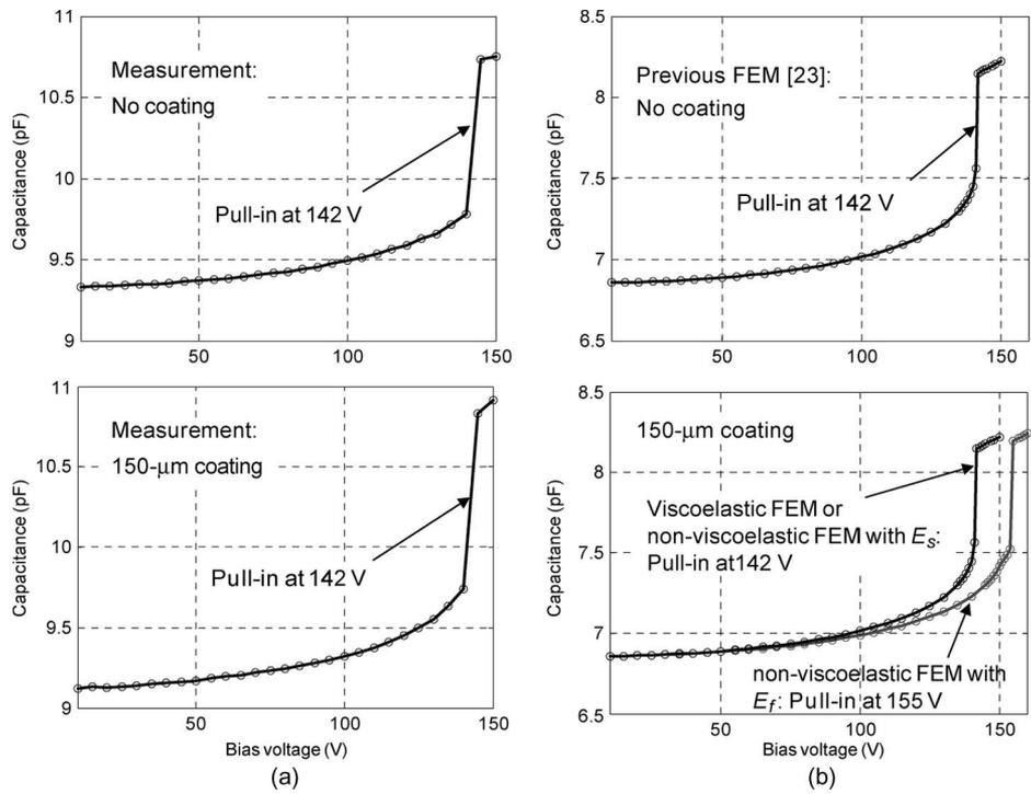
Fig. 5. Static behavior verification: capacitance versus dc bias voltage for the imaging CMUTs: (a) The experimental and the (b) modeling data. The measured capacitance larger than the modeling is due to the parasitics from the electrical interconnections of the experimental setup.
