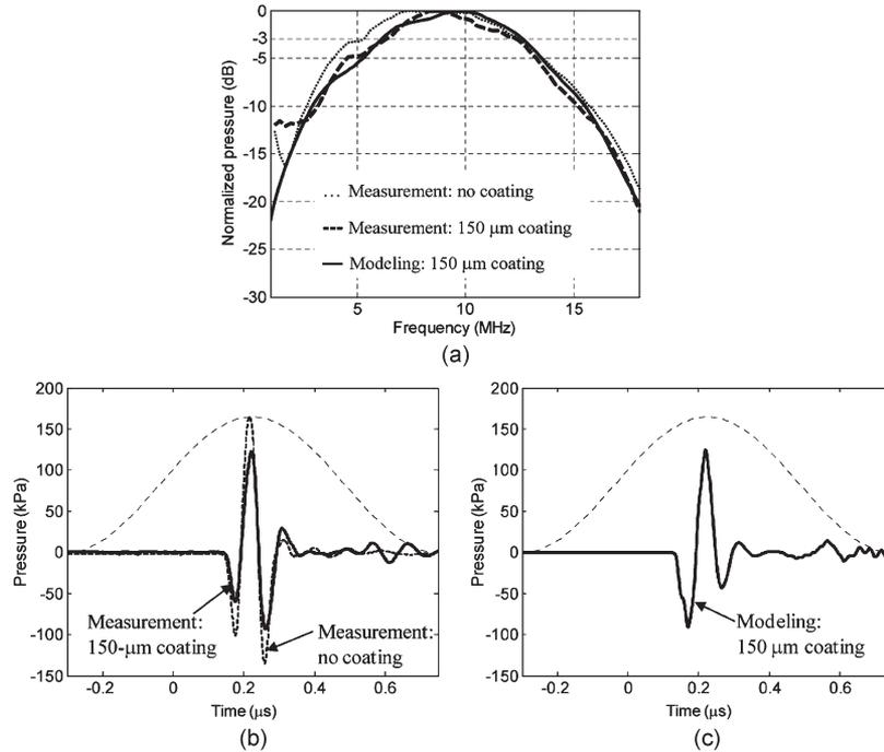
Fig. 8. Comparison between the measurements (with and without the 150  $\mu\text{m}$  of GE RTV 615 coating) and the viscoelastic FEM (with the 150  $\mu\text{m}$  of GE RTV 615 coating) results for imaging CMUTs: (a) the frequency domain and (b) and (c) the time domain. The data were retrieved from the PDMS-water interface.
