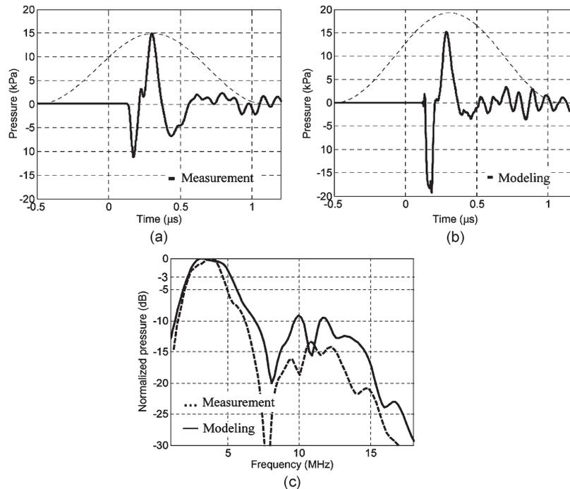
Fig. 10. Comparison between the (a) measurements and the (b) results from the viscoelastic model in the time domain and (c) those in the frequency domain for the HIFU device with a CMUT cell radius of  $70\ \mu\text{m}$  with  $150\ \mu\text{m}$  of GE RTV 615 coating. The data was retrieved from the plate-PDMS interface.
