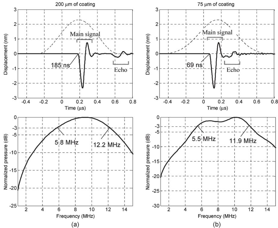
Fig. 6. Viscoelastic FEM results showing the effect of different PDMS coating thicknesses: (a) 200- and (b) 75-μm of GE RTV 615 PDMS coating.  $t = 0$  s corresponds to the beginning of the 50-ns pulse. The data were retrieved from the PDMS-water interface.
