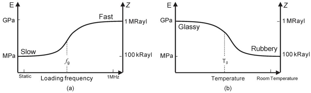
Fig. 1. Viscoelastic curves of PDMS in terms of the Young's modulus and acoustic impedance over (a) loading frequency or (b) temperature based on the theory of time-temperature superposition [7], [8].  $T_g$  and  $f_g$  represent the glass-transition temperature under static loading and the glass-transition loading frequency at room temperature, respectively.
