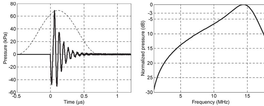
Fig. 9. Results from the nonviscoelastic FEM with  $E_s$  for imaging CMUTs with  $150\ \mu\text{m}$  of GE RTV 615 coating. The data were retrieved from the plate-PDMS interface.  $E_s$  leads to the slower speed of sound, so there was no data from PDMS-water interface before  $1.2\ \mu\text{s}$ .
