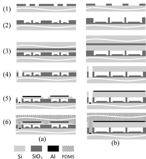
Fig. 2. CMUT device fabrication using wafer bonding technique for (a) imaging CMUTs and (b) HIFU CMUTs. The process flow includes (1) first oxidation and BOE oxide etch, (2) second oxidation and dry etching, (3) wafer bonding, (4) handle wafer and buried-oxide (BOX) removal and etch back for substrate access, (5) top electrode deposition and patterning, and (6) PDMS coating.
