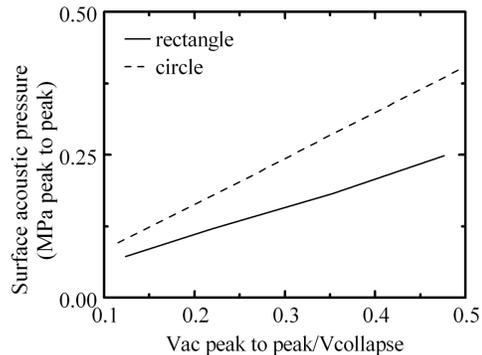
Figure 6: Acoustic output pressure of a circular cell design compared to a rectangular cell design with comparable pull-in voltages and center frequencies.
