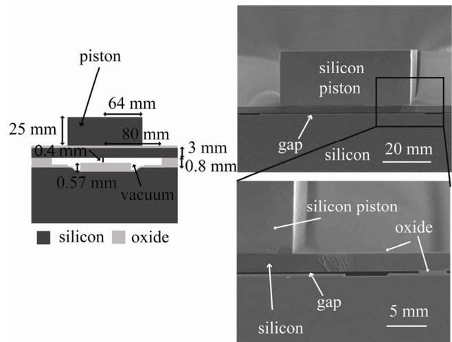
Figure 2: Schematics (a) and SEMs (b) of a circular single cell of a piston CMUT. The transducer is able to produce CW 1 MPa peak to peak output pressure used for the therapeutic ultrasound applications in an 8-element concentric ring array.
