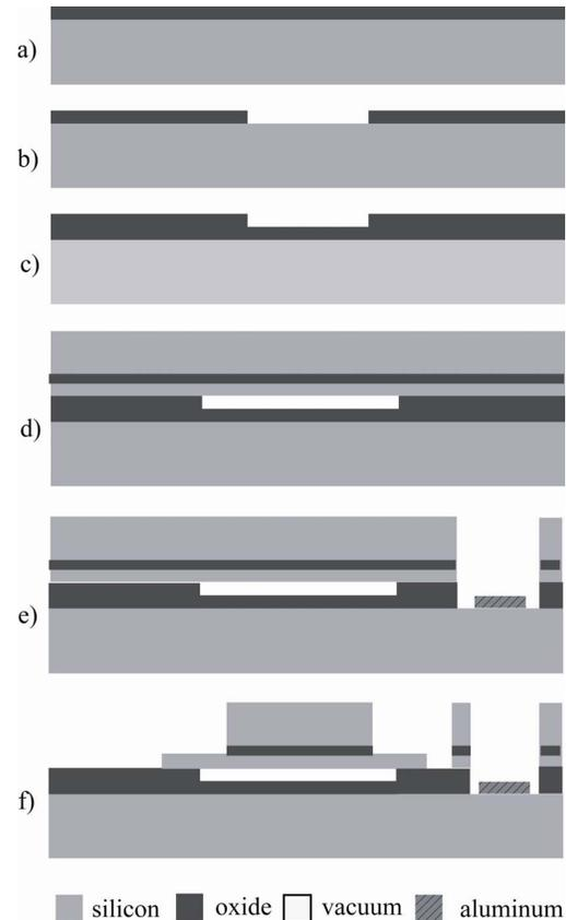
Figure 3: The prime wafer is first oxidized (a) and then etched (b) to form the cavities. A second oxidation (c) forms the insulation layer that protects the device from dielectric breakdown. In the case of a piston device, a double SOI wafer is fusion bonded to the cavity wafer (d) and the handle and buried oxide layer are removed by wet etching.
