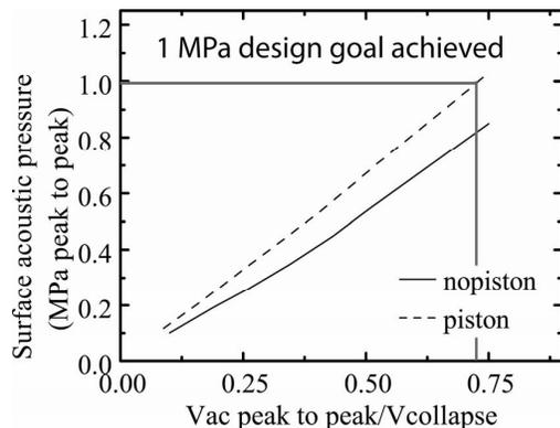
Figure 7: Output pressure of a piston CMUT compared to a non-piston device.
