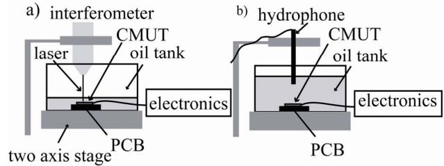
Figure 4: Setups for measuring dynamic displacement (a) and acoustic output pressure (b).
