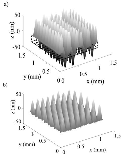
Figure 5: Displacement during steady state operation for a rectangular (a) versus a circular (b) CMUT design.
