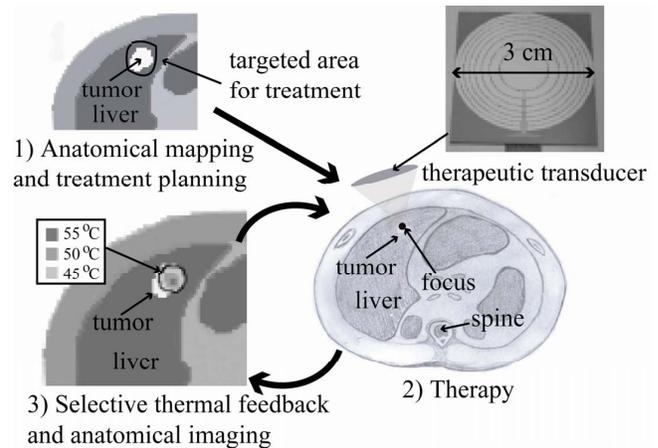
Figure 1: MRI is used to plan the targeted area for treatment around the tumor (1). A CMUT 8-element annular ring array (2) focuses ultrasound to heat and kill cancerous cells; heating constantly monitored with thermal feedback from MRI to adjust the therapy in real-time (3).
