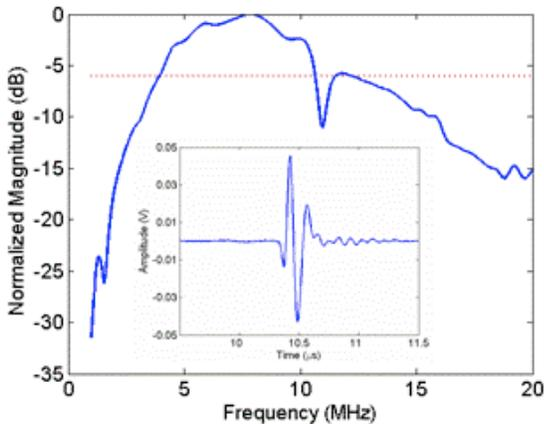
Figure 5. Pulse-echo signal, and corresponding spectrum.
