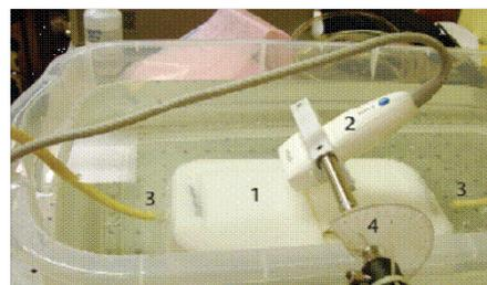
Figure 8. Setup of using a 1D array to obtain five cross-sectional color flow Doppler images of a phantom.
