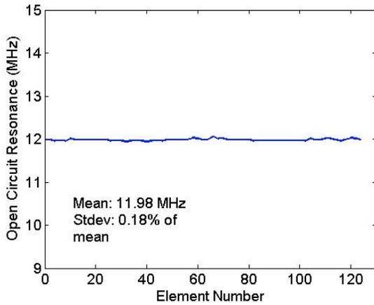
Figure 4. Resonant frequency distribution across a 1D array.
