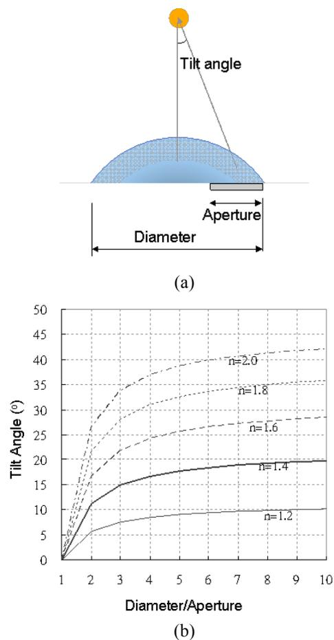
Figure 7. (a) Illustration of off-axis beam steering using an off-centered cylindrical lens. (b) Tilt angle as a function of the ratio of acoustic velocities in the lens material and in water ( $n = v_{\text{water}}/v_{\text{lens}}$ ).
