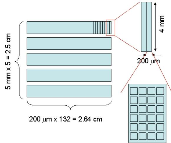
Figure 2. Active array area illustration.
