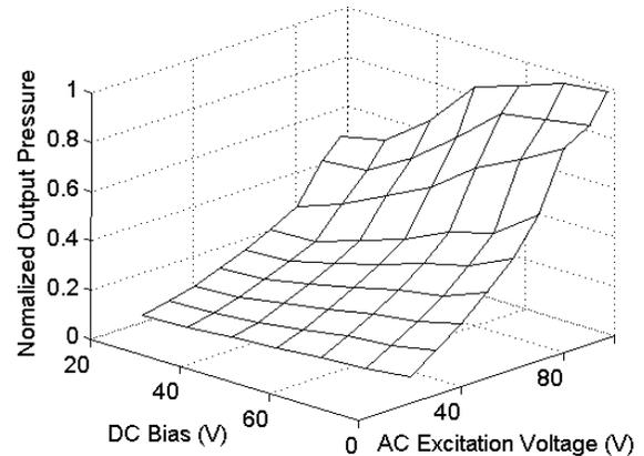
Figure 6. Normalized output pressure as a function of DC bias and AC excitation voltages.
