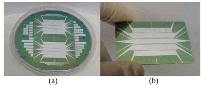
Figure 3. (a) A 4-inch silicon wafer after the completion of fabrication. The center two devices are 5-plane CMUT arrays; the periphery contains test devices. (b) A 5-plane CMUT array diced off from the wafer.
