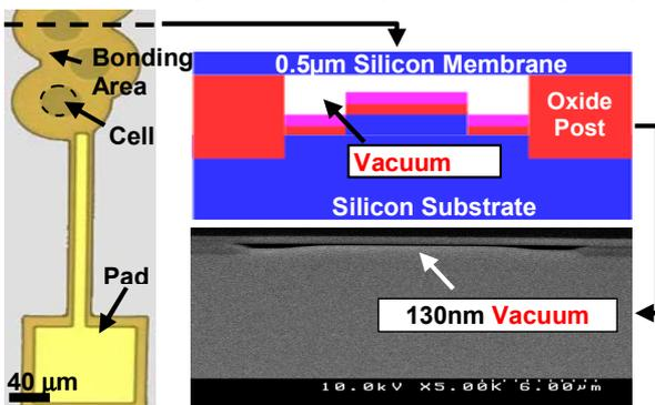
Figure 1: Schematic diagram and cross-sectional SEM of a single cell from the multi-cell CMUT resonator.
