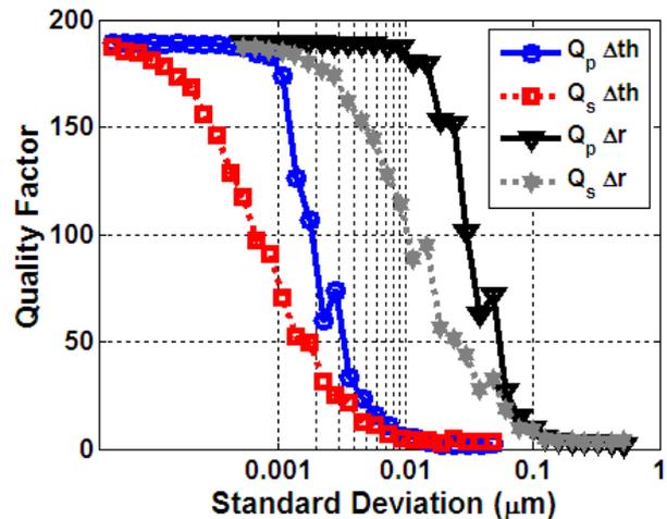
Figure 5: Simulation results showing the effect of process variations on  $Q_s$  and  $Q_p$  assuming the process variation is a normal distribution. 169 CMUT resonators are placed in parallel with mean radius and thickness of 5.3  $\mu\text{m}$  and 0.5  $\mu\text{m}$ , respectively. The standard deviation of the thickness ( $\Delta th$ ) and the radius ( $\Delta r$ ) of the membrane are varied.
