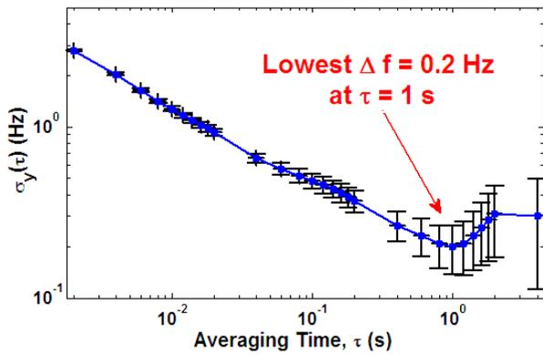
Figure 8: Overlapped Allan deviation calculated from the frequency counter data with a gate time of 2 ms (Stanford Research Systems, Model SRS620, Sunnyvale, CA). The error bars indicate the 1-sigma confidence level.
