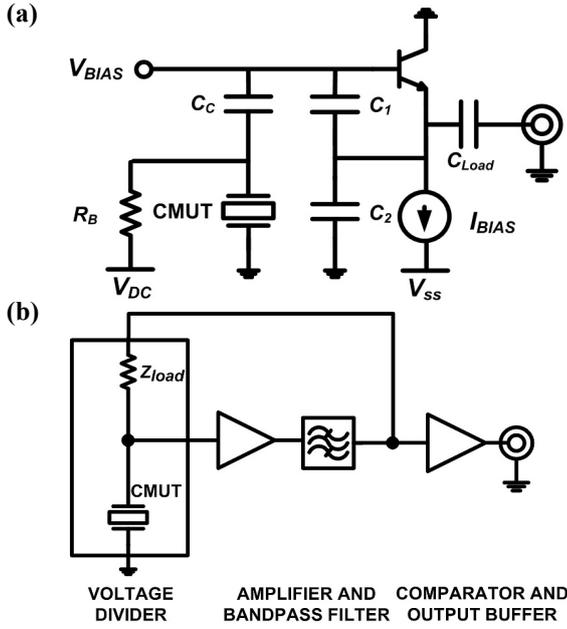
Figure 6: (a) Circuit diagram of the Colpitts oscillator with the bias circuitry of the CMUT resonator shown. (b) Block diagram of the amplifier based oscillator.
