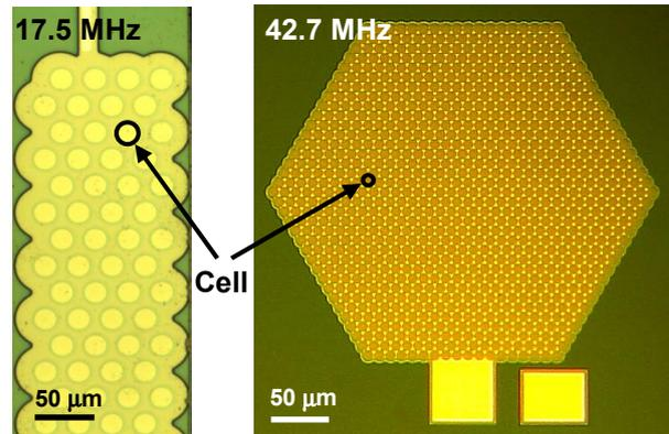
Figure 2: Photographs of the 17.5-MHz and 42.7-MHz CMUT devices with thousand resonator cells.
