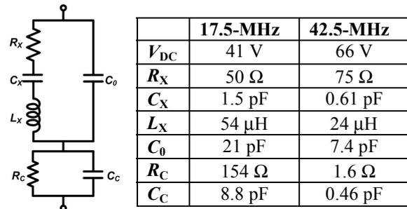
Figure 4: 6-element equivalent circuit model used to fit the input impedance of the CMUT. The values for each components for the two CMUT resonators are shown.
