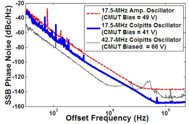
Figure 7: Single side band (SSB) phase noise of the 17.5-MHz amplifier based oscillator, the 17.5-MHz Colpitts oscillator, and the 42.7-MHz Colpitts oscillator, measured using a signal source analyzer (Agilent Technologies, Model E5052B, Palo Alto, CA).
