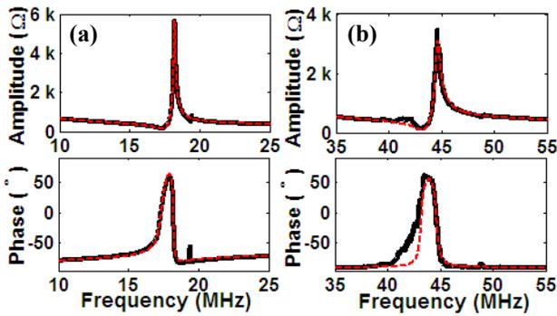
Figure 3: Measured and fitted impedance characteristics of (a) the 17.5-MHz CMUT, (b) the 42.7-MHz CMUT, in air. (Solid line: measurement, dotted lines: fitted).
