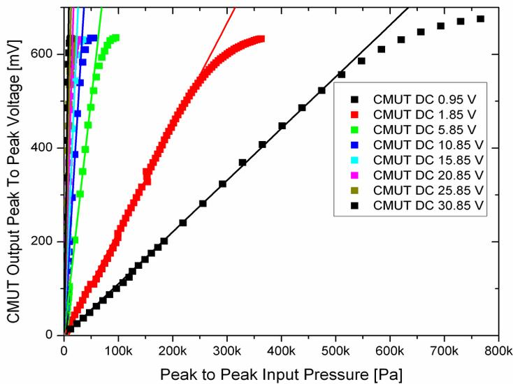
Figure 3. CMUT response as a function of input pressure and CMUT DC bias voltage. Linear fit to find sensitivity of device.
